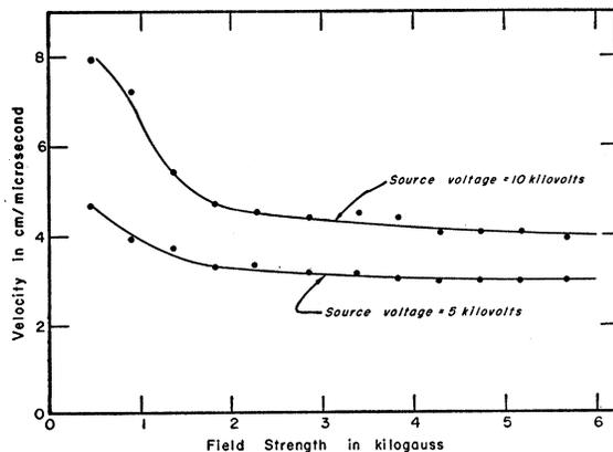
FIG. 7. Velocity vs magnetic field with source current parallel to field.
