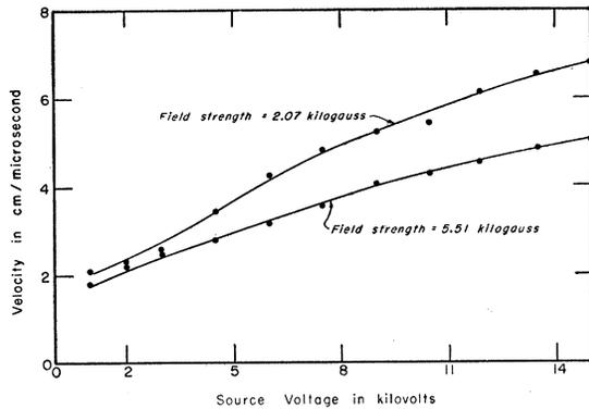
FIG. 4. Velocity vs source voltage with source current parallel to field.
