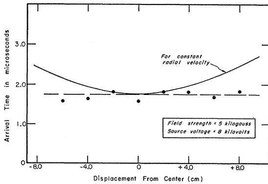
FIG. 1. Profile of the plasma front.
