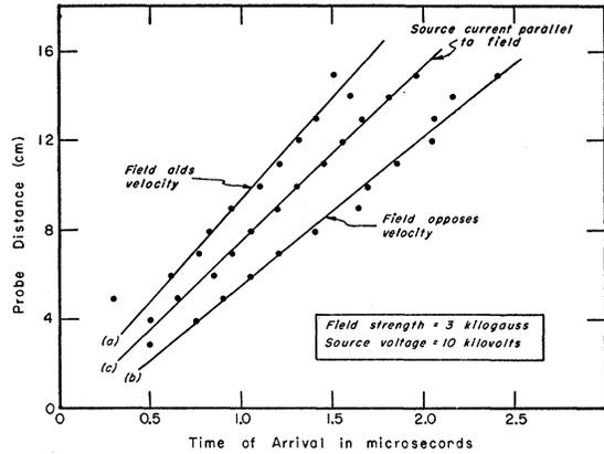
FIG. 2. Arrival time vs probe distance (source voltage 10 kv).
