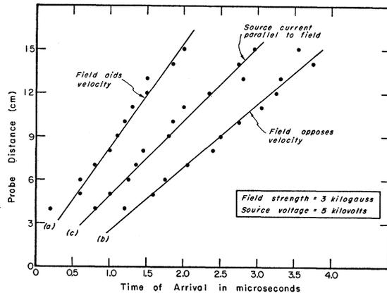
FIG. 3. Arrival time vs probe distance (source voltage 5 kv).
