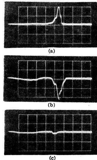
FIG. 9. Probe signals obtained with a polarization detector probe. (a) Probe orientated perpendicular to the field. (b) Probe rotated through 180°. (c) Probe orientated parallel to the field. In all cases the source voltage was 7 kv and the field was 3000 gauss.
