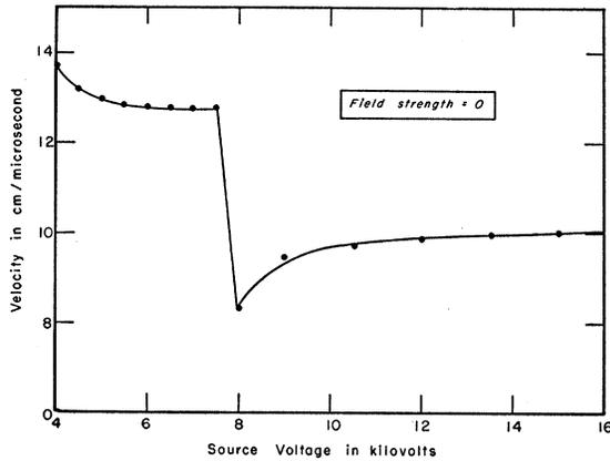
FIG. 6. Velocity vs source voltage at zero magnetic field.
