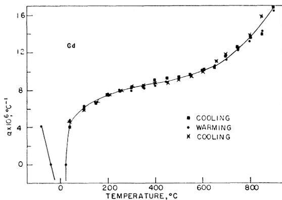
FIG. 7. Thermal expansion coefficient of Gd vs temperature.
