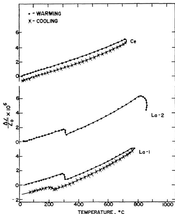
Fig. 2. Relative changes in length of La and Ce vs temperature.
