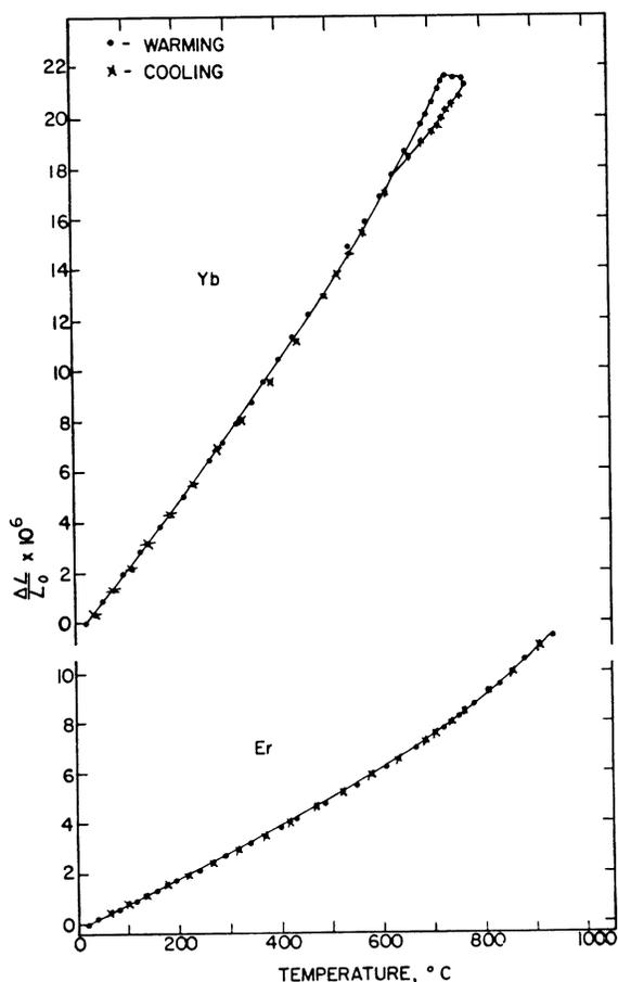
FIG. 10. Relative changes in length of Er and Yb vs temperature.
