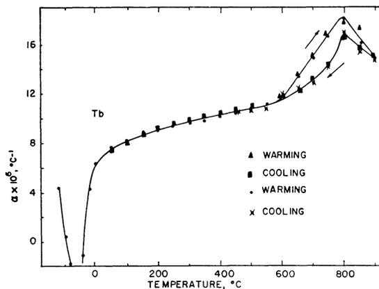
FIG. 8. Thermal expansion coefficient of Tb vs temperature.
