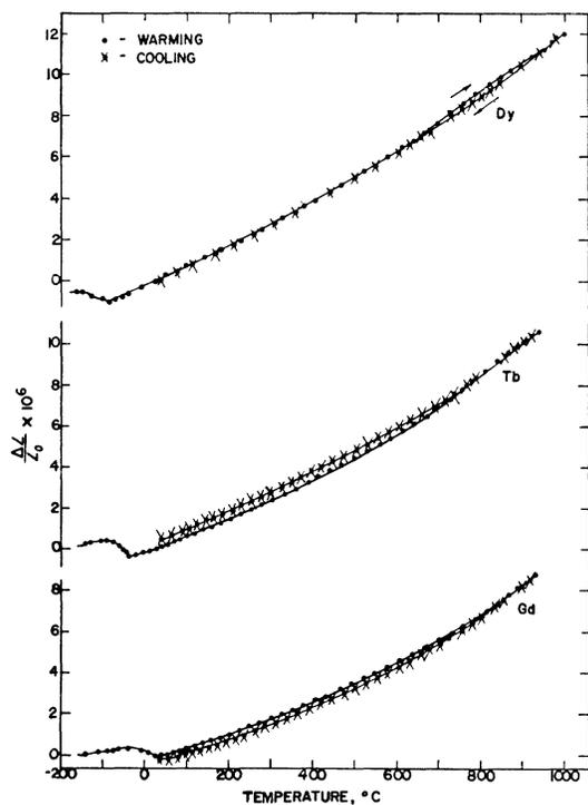
FIG. 6. Relative changes in length of Gd, Tb, and Dy vs temperature.
