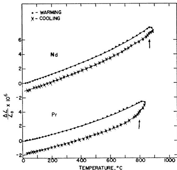
FIG. 4. Relative changes in length of Pr and Nd vs temperature.
