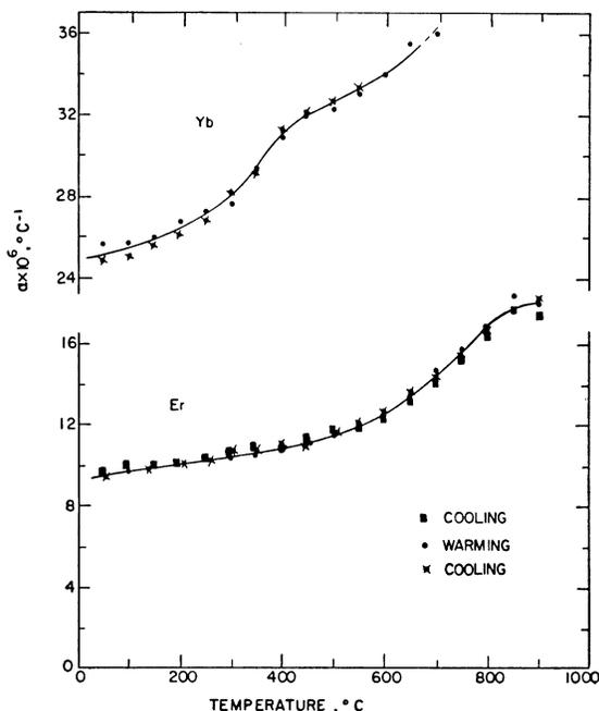
FIG. 11. Thermal expansion coefficients of Er and Yb.
