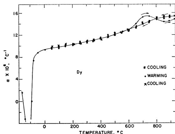
FIG. 9. Thermal expansion coefficient of Dy vs temperature.
