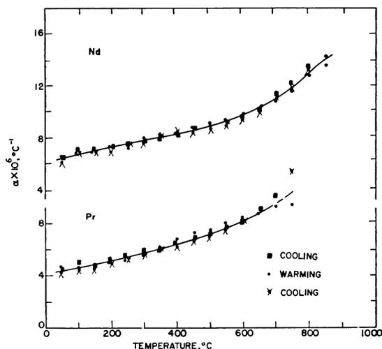
FIG. 5. Thermal expansion coefficients of Pr and Nd vs temperature.
