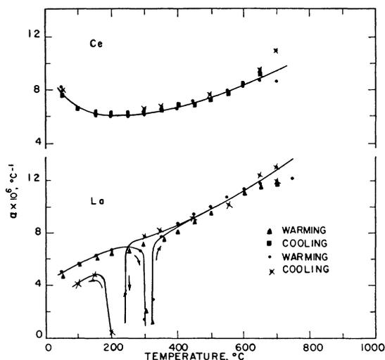
Fig. 3. Thermal expansion coefficients of La and Ce vs temperature.
