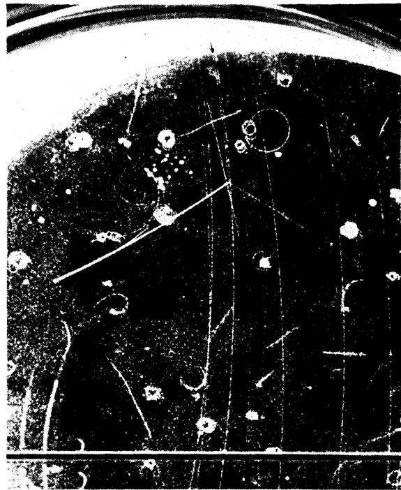
FIG. 6. Diffusion cloud chamber photograph of elastic scattering in deuterium. The incoming beam track is indicated by an arrow. The recoil deuteron comes to rest in the gas.
