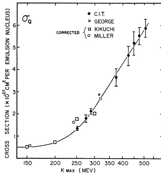
FIG. 2. The cross section per  $Q$  per emulsion nucleus for photostars with 3 or more prongs. The data of Kikuchi has been reduced 2.7 times while Miller's corrected values have been reduced by 30%, the limit quoted for his monitor error. These adjusted values are compared with the work of George and our values. The solid line is a visual fit to the experimental points and implies that the cross section per photon is constant above 300 Mev.
