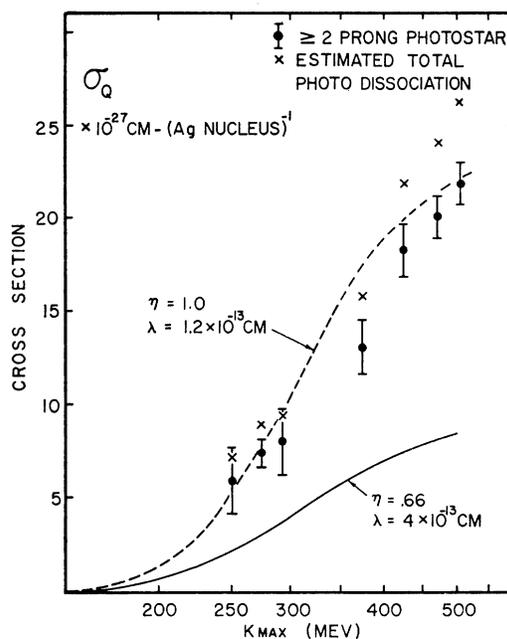
Fig. 3. Photostar cross sections per  $Q$  per equivalent silver nucleus. Star yields, due to photons below the meson threshold, have been subtracted. The solid curve gives the values predicted by the optical model using parameters from other experiments. The dotted curve assumes no nuclear binding and a short mean free path for pions in nuclear matter.
