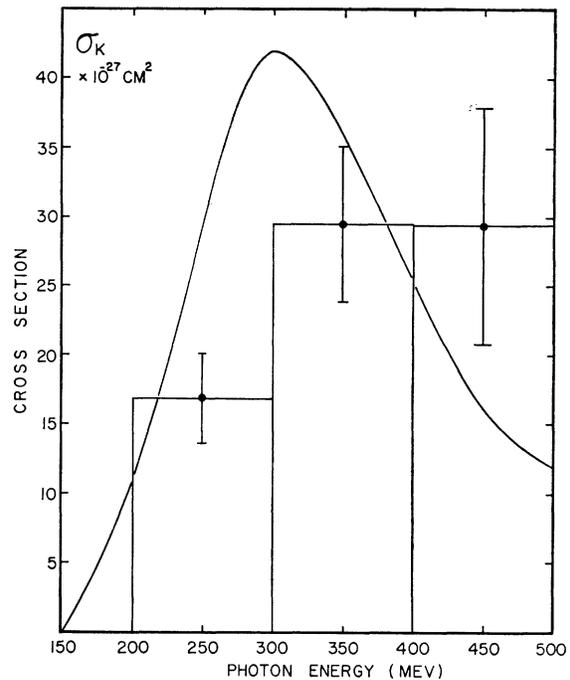
FIG. 5. The photostar cross section per photon per equivalent silver nucleus. The histograms represent the differentiation of the total excitation cross section in Fig. 3. The solid curve is 108 times the photomeson cross section from free nucleons.
