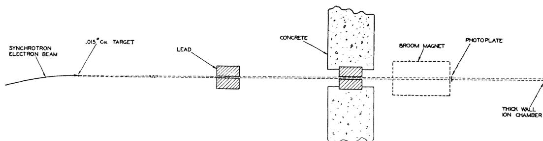
FIG. 1. The location of collimators and broom magnet during exposure.
