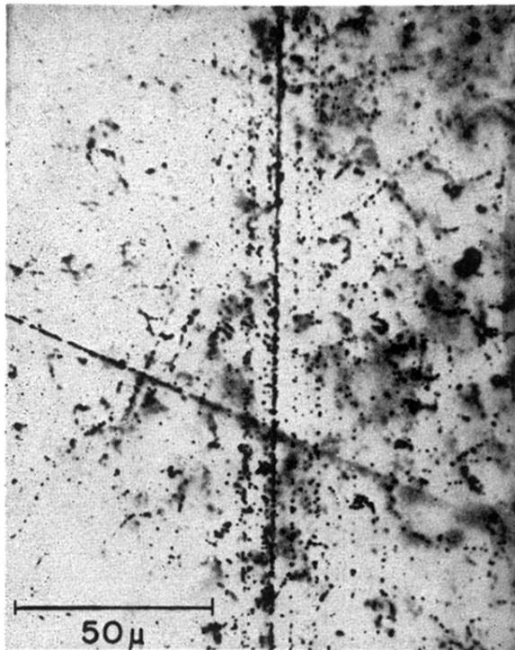
FIG. 3. The shower of Fig. 1, 2.9 cm from the point of interaction. The track of the boron fragment is visible at the core of the shower.
