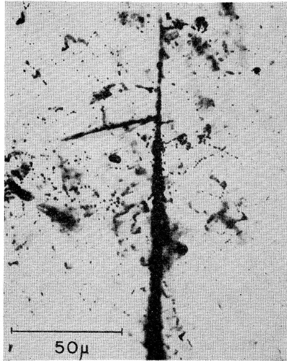
FIG. 1. Photomicrograph of an interaction of a  $(1.4 \pm 0.7) \times 10^{15}$  eV/nucleon nitrogen nucleus in which 110 singly charged shower particles and a boron fragment go on.
