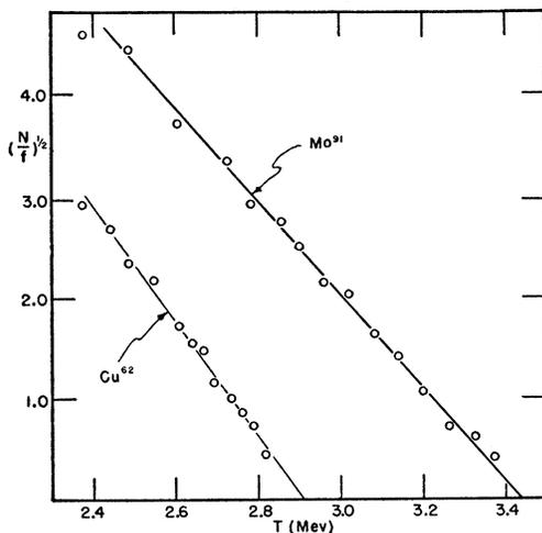
FIG. 1. Kurie plot of the 15-minute positrons from  $\text{Mo}^{91}$ .
