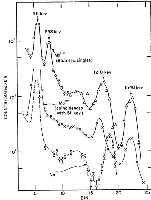
FIG. 2. Pulse-height spectrum of gamma rays from  $\text{Mo}^{91m}$  with a NaI(Tl) crystal. The upper curve is the spectrum of single counts; the middle curve is the gamma spectrum which is in coincidence with annihilation radiation.
