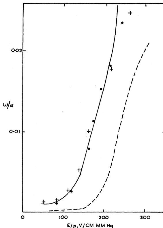
FIG. 4.  $(\omega/\alpha)$ ,  $(E/p)$  curves for copper electrodes in hydrogen after various treatments. — Llewellyn Jones<sup>16</sup>; ••• Llewellyn Jones and Davies<sup>13</sup>; +++ present work.
