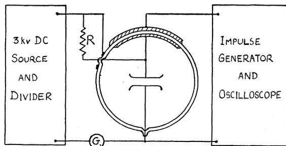
FIG. 1. Schematic diagram of discharge tube and circuit.
