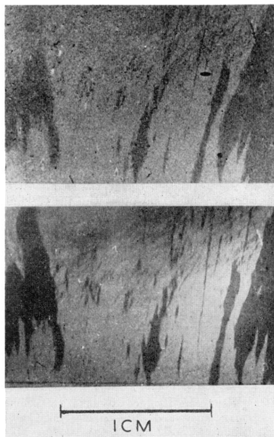
FIG. 1. Photographs of the domain structure of a transparent NiFe film in the same magnetic state, taken (upper) with the Kerr magneto-optic reflection technique and (lower) with the transmission method utilizing the Faraday effect.
