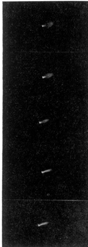
FIG. 5. Kerr-cell photographs taken under the same circumstances as Fig. 3, except that magnetic fields (geometry as shown in Fig. 2, with field out of paper) of values 600, 1200, 1800, 2400, and 3000 gauss have been applied. Note the squeezing effect in the vertical direction and the consequent tendency to form an elongated hairpin-like loop.
