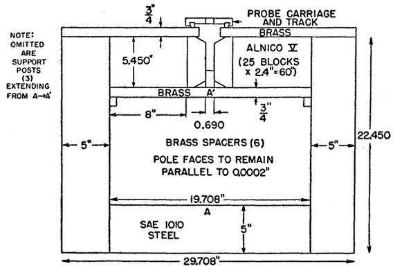
FIG. 4. Vertical section through the magnet which furnishes the steady field. The field strength is approximately 8500 gauss.
