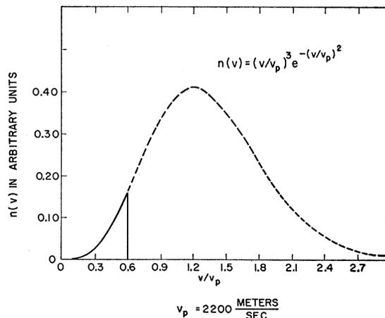
FIG. 2. The solid curve shows roughly the velocity spectrum of the neutron beam reflected from the mirror at  $\theta = 0.005$  radian (17'). The broken line shows the approximate spectrum of neutrons in the original beam.
