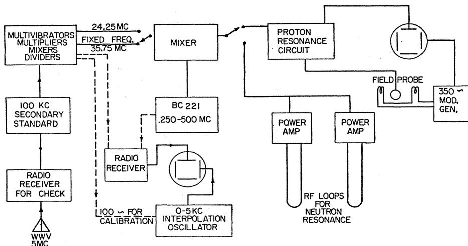
Fig. 6. Block diagram of the signal generator showing the alternate channels to the neutron loops and the magnetic field probe.
