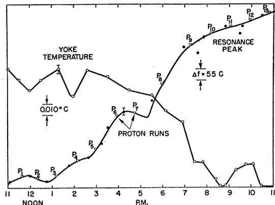
FIG. 10. Curve of changes in yoke temperature and average neutron frequency as a function of time for a typical run. Abscissae are in arbitrary units of temperature and frequency.
