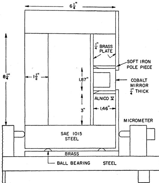
FIG. 3. Cross section of polarizing magnetic mirror, showing mounting arrangement.
