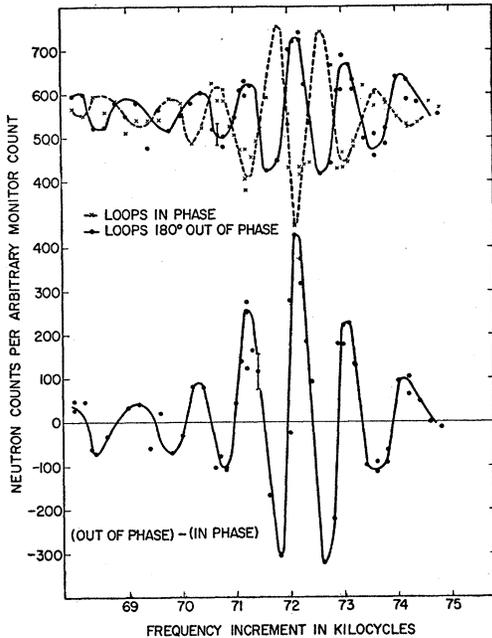
FIG. 8. Upper curves show neutron counts as a function of frequency with the loops in phase and  $180^\circ$  out of phase respectively. Lower curve shows the count difference between the two upper curves as a function of frequency.
