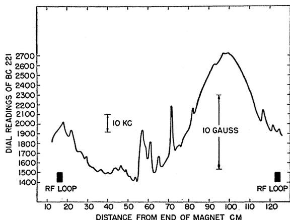
FIG. 5. Plot of the magnetic field along the beam trajectory.
