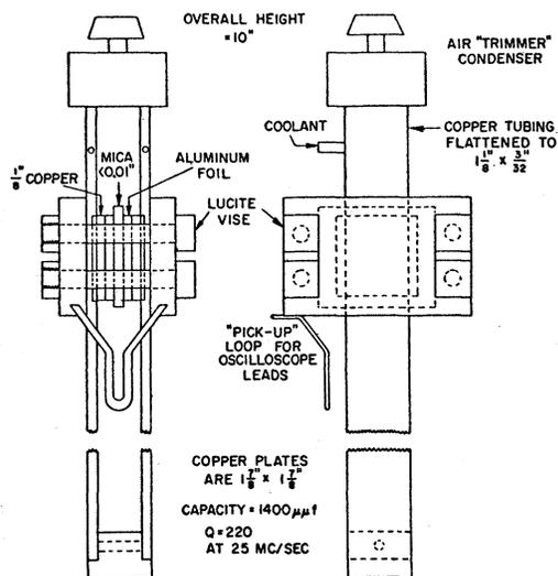
Fig. 7. Sketch of one of the neutron "flopping" loops. The loop was tuned for a resonance at 24.7 Mc/sec.
