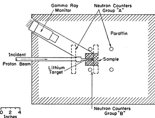
FIG. 1. The experimental arrangement.
