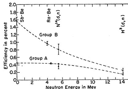
FIG. 2. Efficiency calibration for the two groups of neutron counters.
