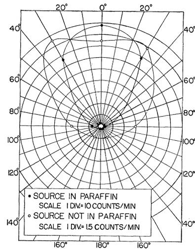
FIG. 3. Directional selectivity of low-energy neutron detector measured with a Ra-Be source.
