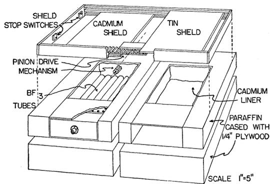
FIG. 2. Low-energy directional neutron detector, *D-2*, with five  $BF_3$  counters in each half-section.
