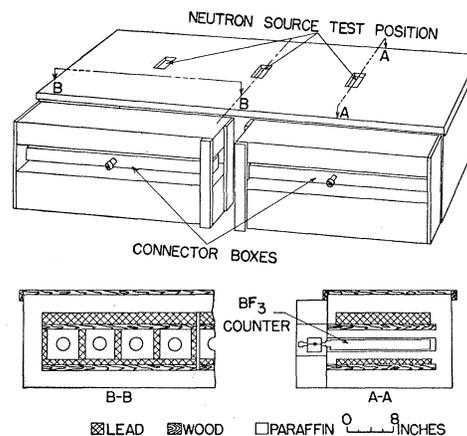
FIG. 1. Lead-paraffin neutron monitor, D-1, with eight  $BF_3$  counters.
