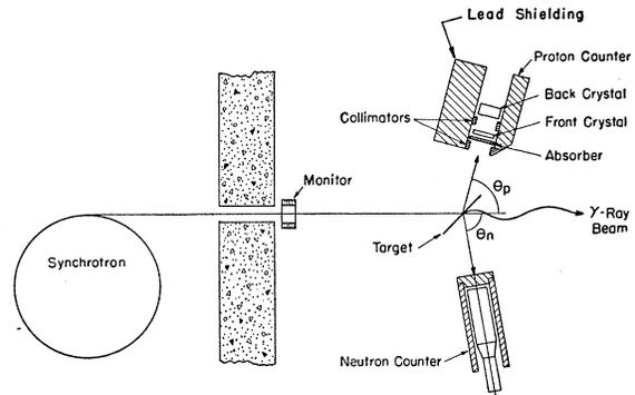
FIG. 1. The geometrical arrangement of the apparatus. The proton angle was kept fixed; the angle of the neutron counter was varied. The cross-hatching surrounding both counters indicates lead shielding.
