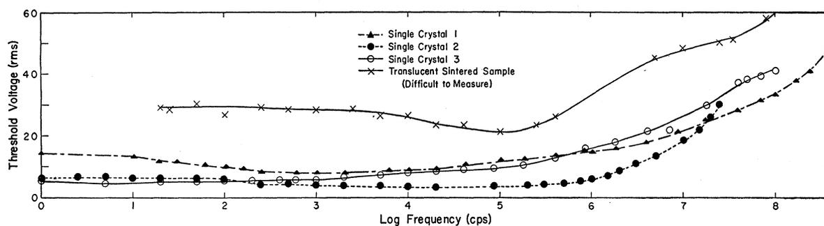
FIG. 1. Voltage necessary to produce threshold electroluminescence ( $V_0$ ) vs logarithm of frequency for four ZnS samples.
