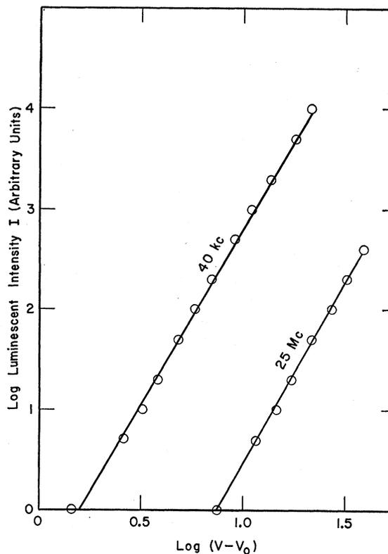
FIG. 2. Time-average electroluminescent intensity ( $I$ ) vs voltage above the threshold ( $V - V_0$ ) for one ZnS single crystal measured at two frequencies.
