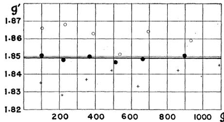
FIG. 1. Plot of  $g'$  vs intensity of magnetization for cobalt. Open circles are values obtained for General Motors rod. Crosses are values obtained for International Nickel Company rod. Solid circles obtained by averaging, for each value of the magnetizing current used, the  $g'$  and  $g$  values for the two rods.
