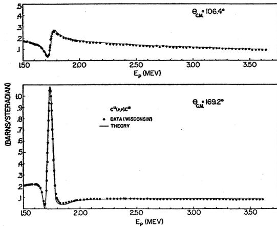
FIG. 6. The  $C^{12}(p,p)C^{12}$  center-of-mass differential cross section vs bombarding energy. The points represent the Wisconsin data and the solid lines represent the theoretical fit obtained by using the phase shifts of the present analysis.
