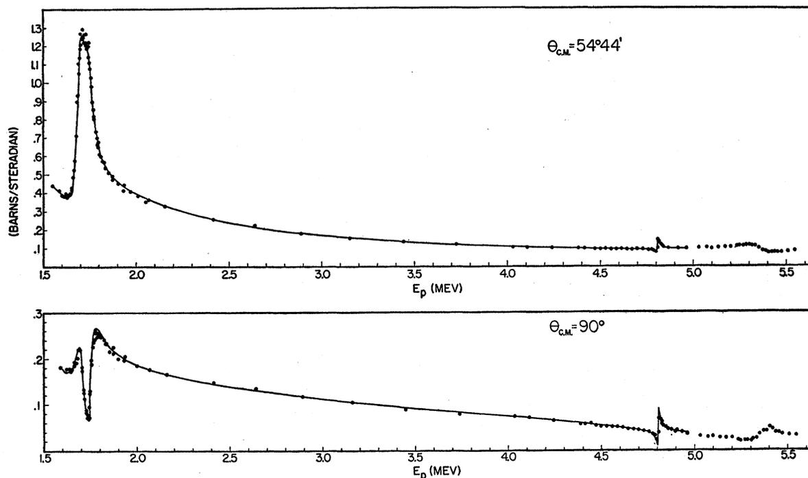
FIG. 4. The C<sup>12</sup>(*p*,*p*)C<sup>12</sup> center-of-mass differential cross section *vs* bombarding energy at two forward angles. The solid line indicates the theoretical fit to the data.
