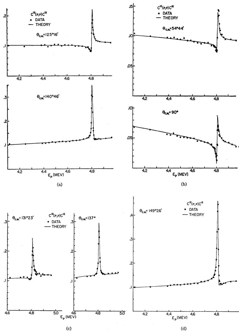
FIG. 1. The  $C^{12}(p,p)C^{12}$  center-of-mass differential cross section (in barns/steradian) vs bombarding energy at the seven angles observed. The data points are solid circles, while the solid line indicates the fit of the theory to these data. The narrow anomaly at 4.808 Mev is the fourth excited state of  $N^{13}$ , and its assignment is  $5/2^+$ . The behavior of the off-resonance cross section is due to the presence of a  $3/2^+$  resonance at 5.37 Mev.
