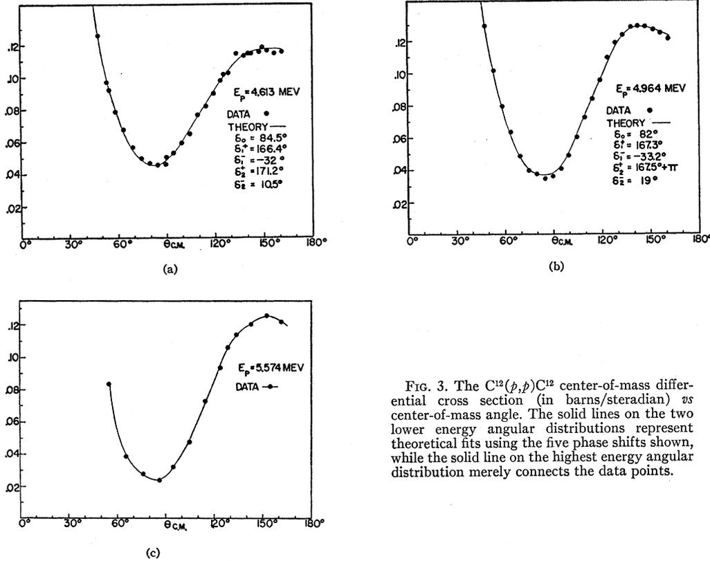
FIG. 3. The  $C^{12}(p,p)C^{12}$  center-of-mass differential cross section (in barns/steradian) vs center-of-mass angle. The solid lines on the two lower energy angular distributions represent theoretical fits using the five phase shifts shown, while the solid line on the highest energy angular distribution merely connects the data points.
