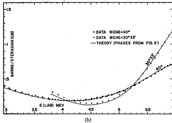
Fig. 5. Excitation curves for  $\alpha$ - $\alpha$  scattering in the energy region 3 to 6 Mev, at four scattering angles. The differential cross section in the c.m. system is plotted *versus* the laboratory energy. The smooth curves are the cross sections calculated from the phase shifts shown in Fig. 6.
