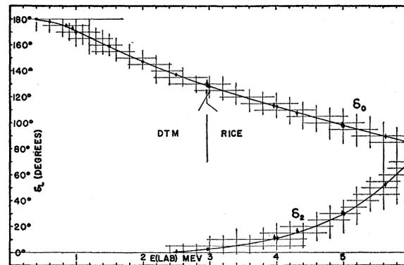
Fig. 6.  $S$ - and  $D$ -wave phase shifts for  $\alpha$ - $\alpha$  scattering in the energy region 0.3 to 6 Mev. Included are the phase shifts of reference 5. Arbitrary smooth curves have been drawn through the data points.
