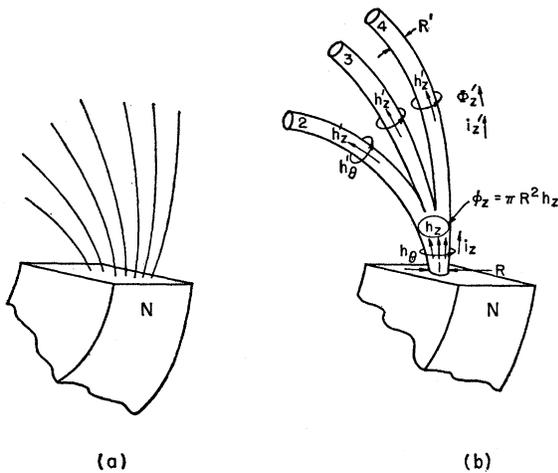
FIG. 3. (a) Magnetic field configuration before any discharge occurs. (b) Postulated magnetic field and current configurations after  $i_z$  currents have gathered both plasma and  $h_z$  field lines into discrete tubes or filaments.
