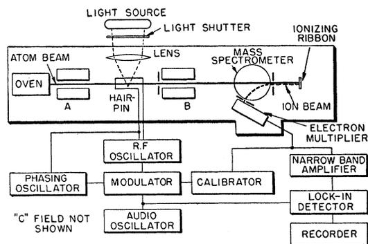
Fig. 1. Schematic drawing of the apparatus.
