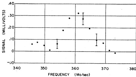
FIG. 9. The  $F=3$  to  $F=2$  transition of  $\text{Rb}^{85}$  in the  $5P_{3/2}$  state.
