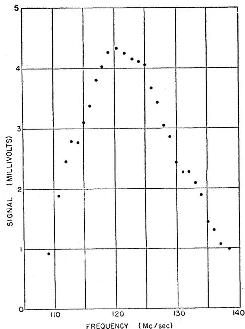
FIG. 7. The  $F=4$  to  $F=3$  transition of Rb<sup>85</sup> in the  $5P_{\frac{1}{2}}$  state.
