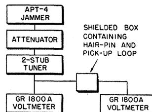
FIG. 3. Hairpin calibration arrangement.
