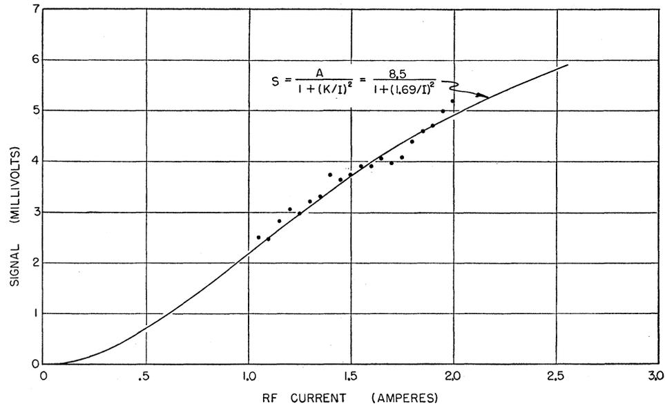
FIG. 6. Signal vs rf current at 65.0 Mc.
