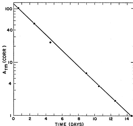
FIG. 1. A plot of  $A_{\text{Tm}}(\text{corr})$  vs time, to give Er<sup>172</sup> half-life.
