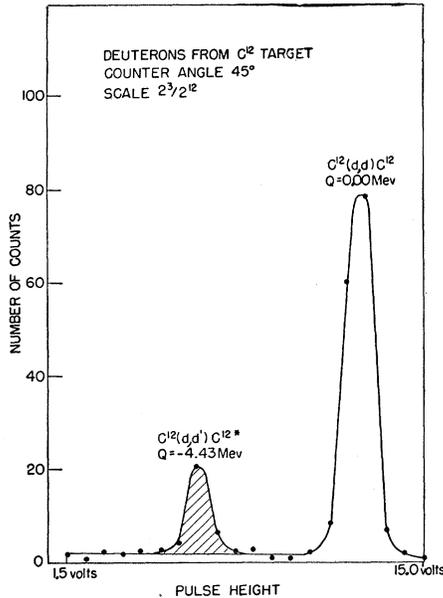
FIG. 5. Scattered deuteron energy spectrum from deuteron bombardment of C<sup>12</sup> target.
