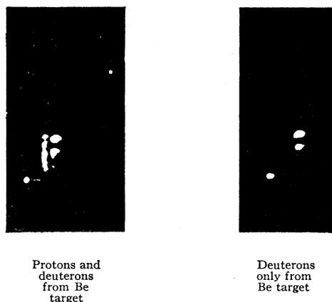
FIG. 8. Photographs of oscilloscope face showing separation of scattered protons and deuterons resulting from deuteron bombardment of Be<sup>9</sup>. In the first photograph, protons are to the left; deuterons are to the right. In the second photograph, only deuterons are shown.
