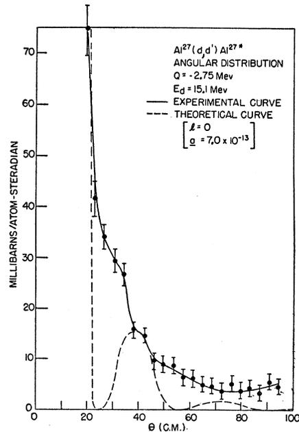
FIG. 15. Comparison of the  $Al^{27}(d,d')Al^{27*}$  ( $Q = -2.75$  Mev) angular distribution with the nuclear interaction theory.
