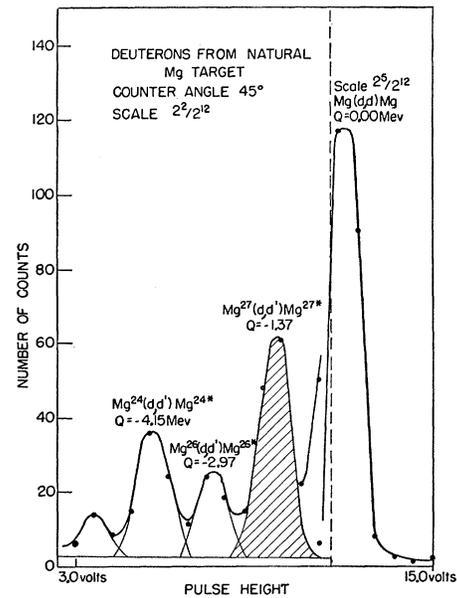
FIG. 6. Scattered deuteron energy spectrum from deuteron bombardment of natural Mg target.
