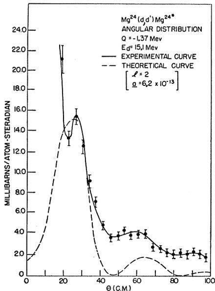
FIG. 13. Comparison of the  $Mg^{24}(d,d')Mg^{24*}$  angular distribution with the nuclear interaction theory.
