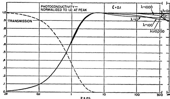
FIG. 6. Photoconductivity-absorption curve,  $\xi = 0.1$ ,  $\lambda = 0.1$  to 10 000.
