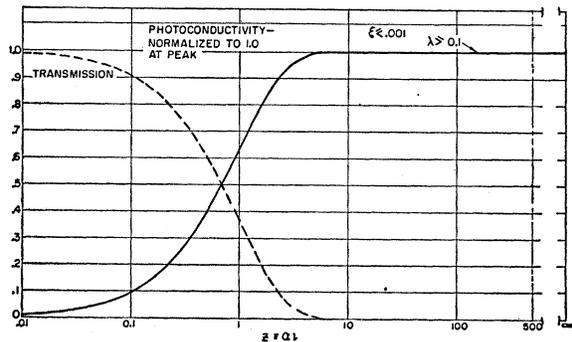
FIG. 5. Photoconductivity-absorption curve,  $\xi \pm 0.001$ ,  $\lambda \geq 0.1$ .
