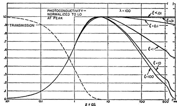
FIG. 3. Photoconductivity-absorption curve,  $\lambda = 100$ ,  $\xi = 0.01$  to 100.
