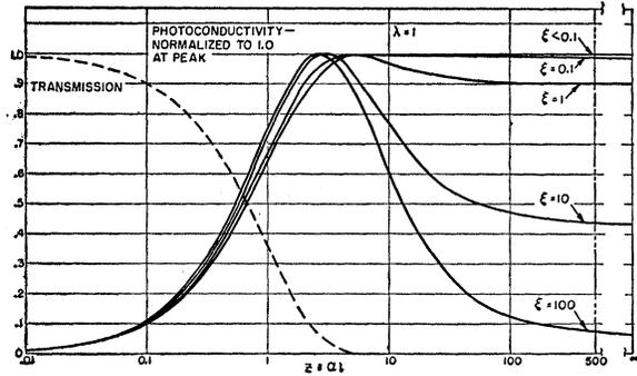
FIG. 2. Photoconductivity-absorption curve,  $\lambda = 1$ ,  $\xi = 0.01$  to 100.
