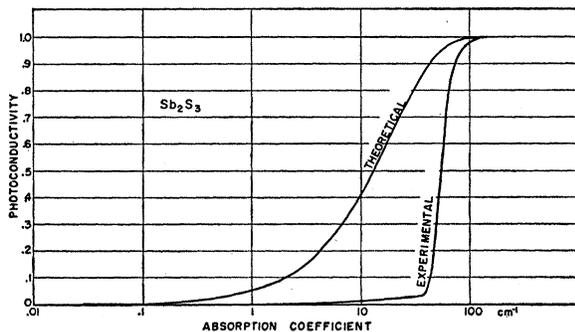
FIG. 9. Photoconductivity-absorption curves for antimony sulfide.
