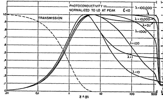
FIG. 7. Photoconductivity-absorption curve,  $\xi = 10$ ,  $\lambda = 0.1$  to 100 000.
