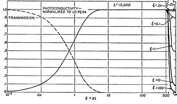
FIG. 4. Photoconductivity-absorption curve,  $\lambda = 10,000$ ,  $\xi = 0.01$  to 100.
