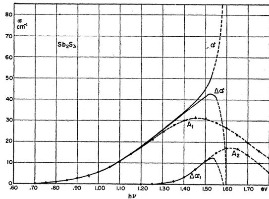
FIG. 10. Low-energy tail of absorption curve for antimony sulfide.  $\alpha$ —experimental absorption curve;  $\Delta\alpha$ —difference between experimental and theoretical curves;  $A_1$ —first absorption band;  $\Delta\alpha_1$ —difference between  $\Delta\alpha$  and  $A_1$  curves;  $A_2$ —second absorption band.
