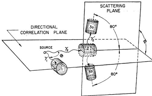
FIG. 4. Geometry of the polarization-directional correlation arrangement.
