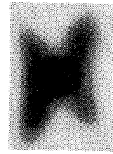
FIG. 19. Deposits obtained when a \{110\} silver plane is sputtered with 100-ev Hg ions
