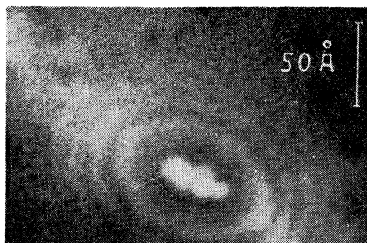
FIG. 11. Helium-ion image of a 011 plane of a tungsten tip with 1000 Å radius, after 10-sec exposure to 500 Mv/cm. Dissolution of 011 lattice planes was halted by lowering the field to 375 Mv/cm, and the picture was taken at this field.
