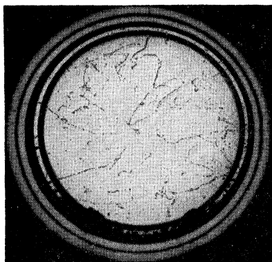
FIG. 1. Tracks of electrons produced by gamma rays from a 100-mC radium beryllium source placed 8 in. from the center of a bubble chamber 1 in. in diameter filled with liquid ethylene at -18^{\circ}\text{C} . The density of the liquid is about 0.5\text{ g/cm}^3 . The duration of the light flash is 5 msec and the flash occurred 3 msec after the expansion was initiated.
