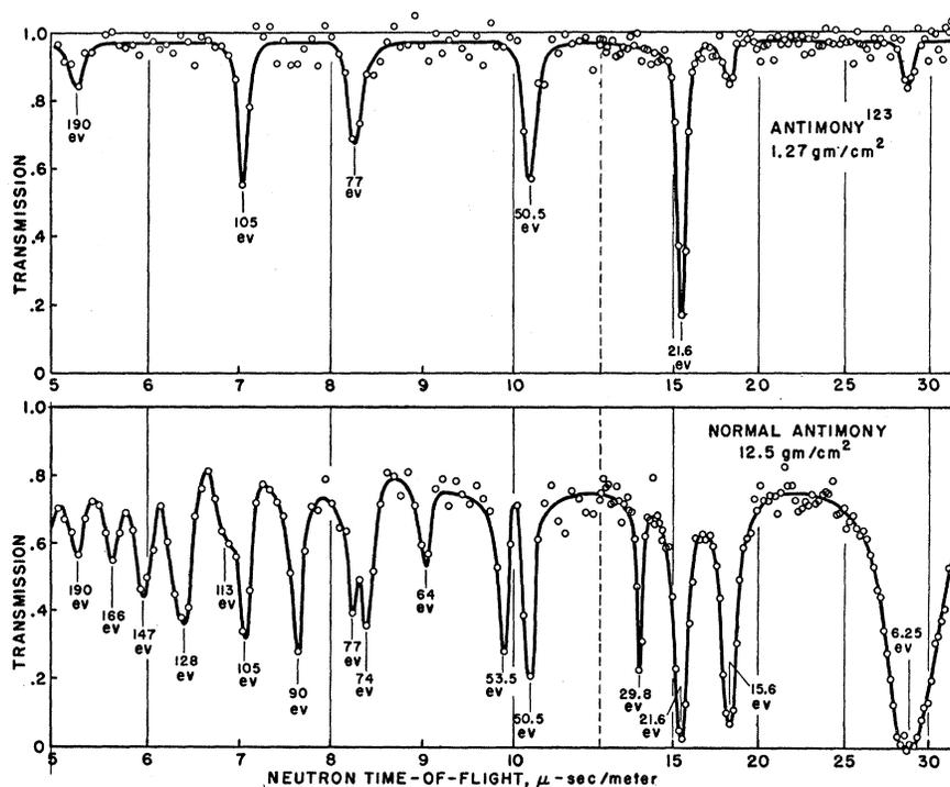
FIG. 1. The neutron transmission of normal antimony and  $\text{Sb}^{123}$ . The data were obtained with a resolution of  $0.12 \mu\text{sec/m}$  for energies greater than 35 eV and about  $0.35 \mu\text{sec/m}$  at the lower energies.
