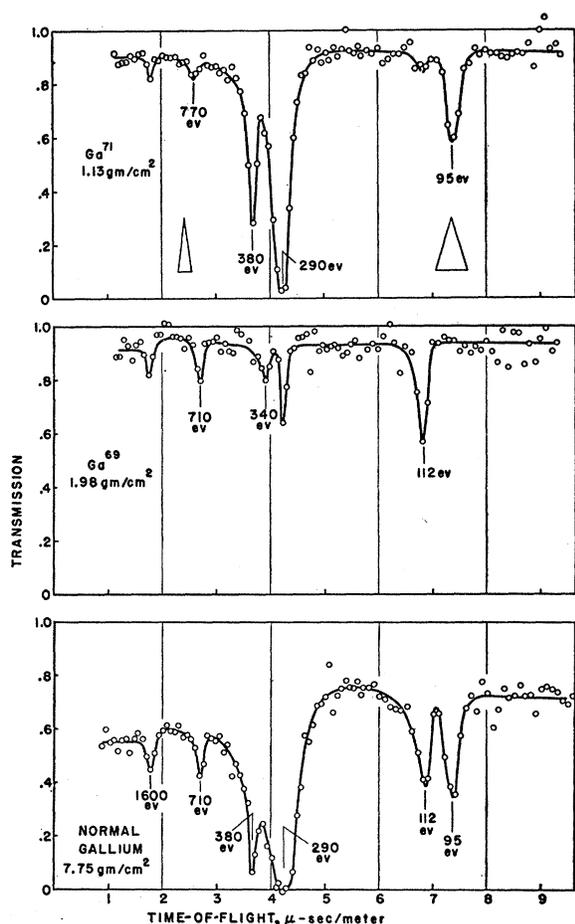
FIG. 5. Neutron transmission of normal gallium and its isotopes as obtained with a resolution of  $0.14 \mu\text{sec/m}$ .
