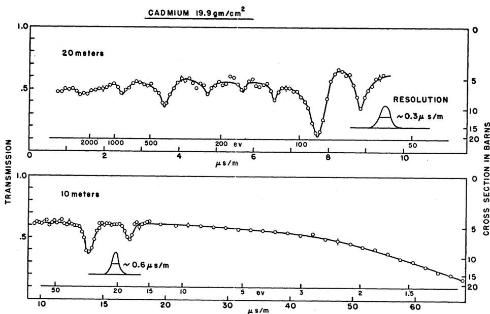
FIG. 7. Neutron transmission of cadmium as a function of time of flight.
