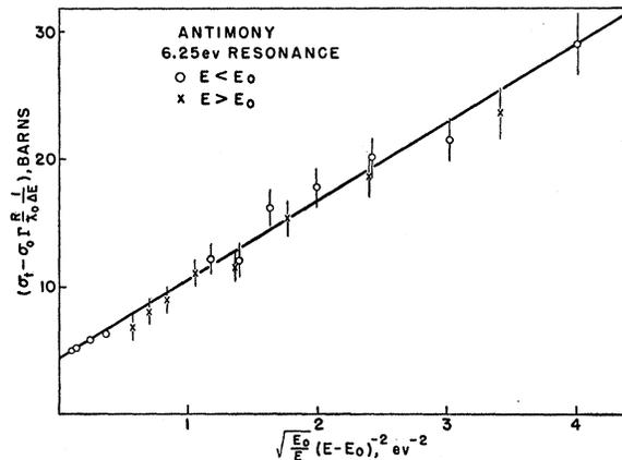
FIG. 3. Wing analysis of the 6.25-ev resonance in  $\text{Sb}^{121}$ . The slope of the straight line gives  $\sigma_0 \Gamma_0^2 = 24.6$  b-ev<sup>2</sup> for normal antimony or 43 b-ev<sup>2</sup> referred to  $\text{Sb}^{121}$ . The Z-intercept gives  $R = 0.59 \times 10^{-12}$  cm.
