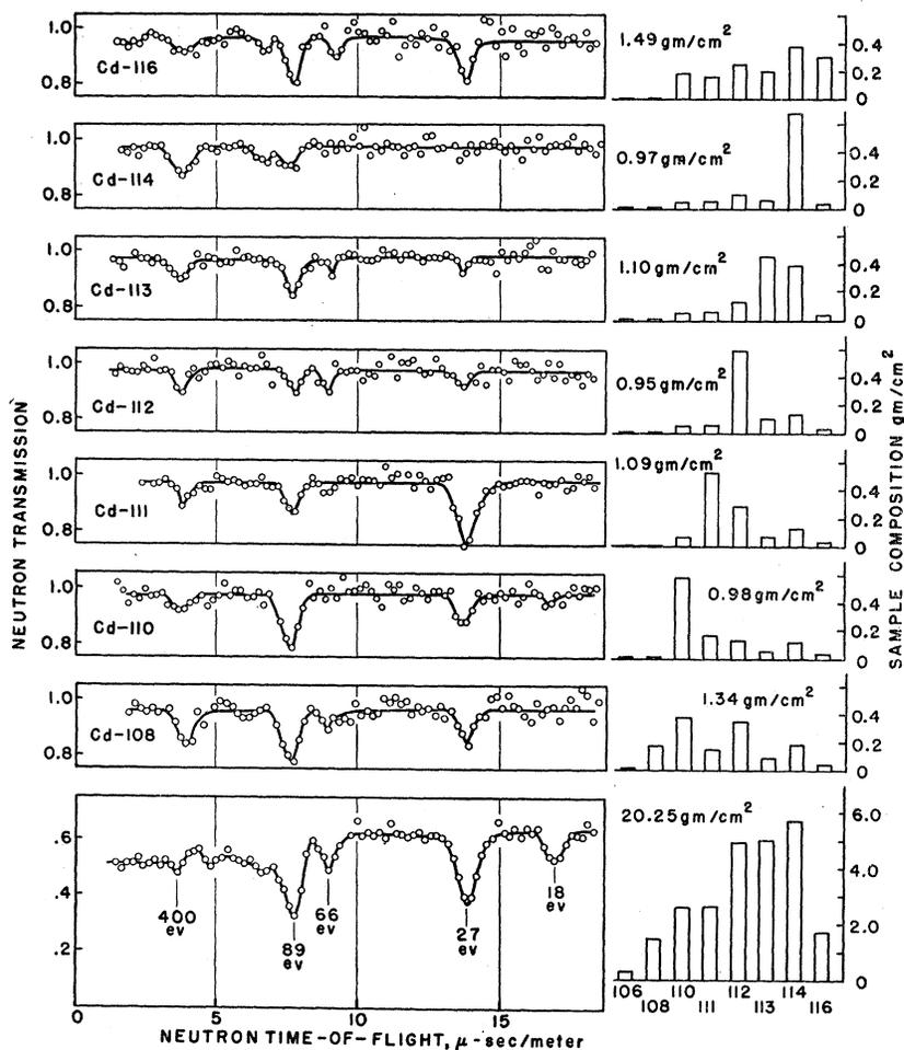
FIG. 8. Neutron transmission of the separated isotopes of cadmium and the transmission of normal cadmium.
