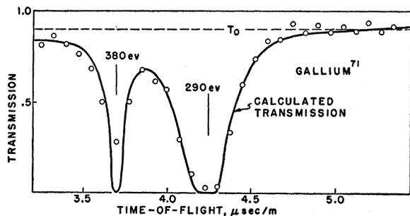
FIG. 6. Comparison of the calculated transmission, using the parameters given in Table III, and the experimentally measured transmission in the vicinity of the 290- and 380-ev resonances of  $\text{Ga}^{71}$ .
