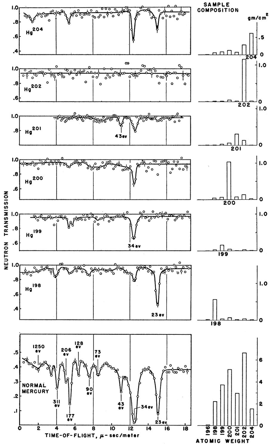
FIG. 9. Neutron transmission of separated isotopes of mercury and the transmission of normal mercury. The resolution used was about 0.3  $\mu$ sec/m.
