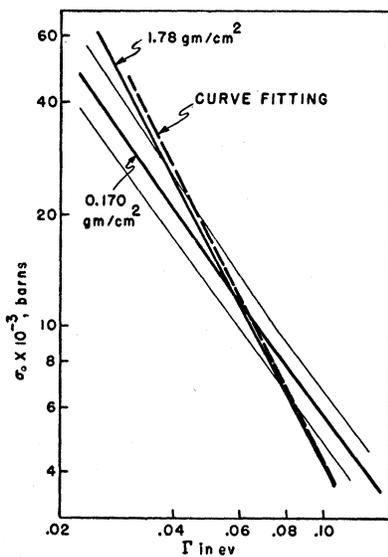
FIG. 2. Analysis of the 6.25-ev resonance in Sb<sup>121</sup>. The heavy solid lines were obtained from area data and the heavy dashed line was calculated from the value of  $\sigma_0\Gamma^2$  obtained by curve fitting. The fine solid lines indicate the magnitude of the errors associated with the 0.170 g/cm<sup>2</sup> data.
