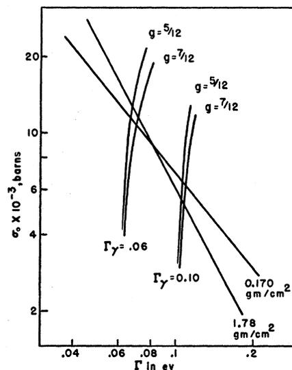
FIG. 4. Analysis of the 15.6-ev resonance in  $\text{Sb}^{121}$ , illustrating a convenient technique of obtaining resonance parameters from area data for assumed values of  $\Gamma_\gamma$ .
