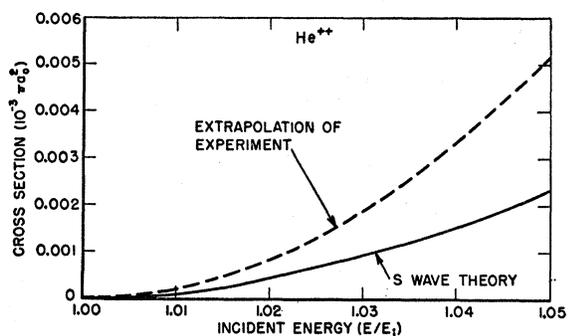
FIG. 3. Comparison of the calculated  $S$ -wave cross section with a quadratic extrapolation of the experimental curve for the double ionization of helium.
