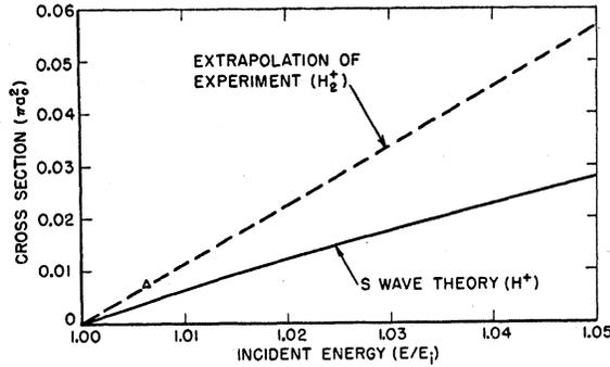
FIG. 1. Comparison of the calculated  $S$ -wave cross section with a linear extrapolation of the experimental curve for the ionization of hydrogen.
