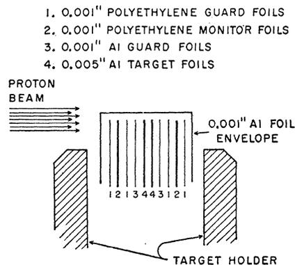
FIG. 1. Schematic target assembly for circulating cyclotron beam bombardments.
