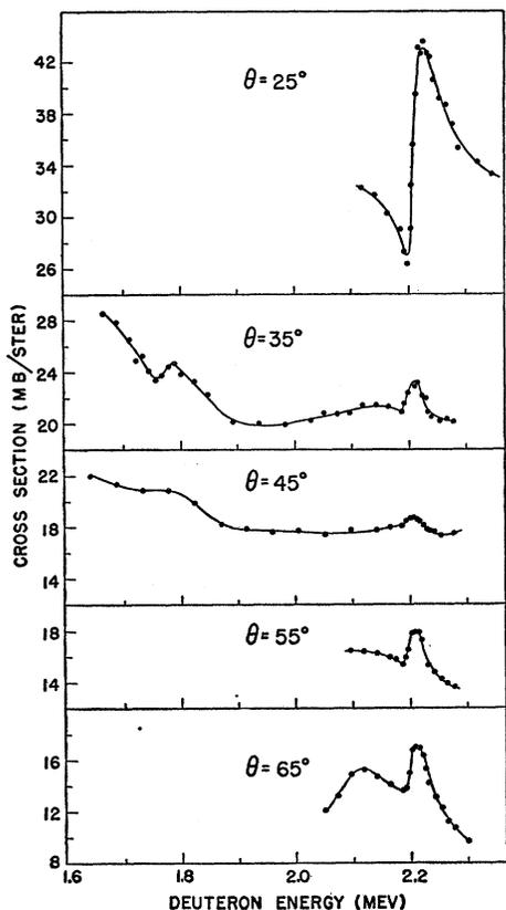
FIG. 6. Excitation curves for the  $C^{13}(d,\alpha)B^{11}$  (ground state) reaction as a function of the bombarding energy in the vicinity of the 2.20-Mev resonance at 6 observation angles in the forward directions. The foil target was used and the energy scale is uncorrected for target thickness.
