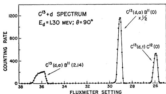
FIG. 1. Momentum profile of the  $\alpha$  particles and tritons from the deuteron bombardment of  $C^{13}$  at an energy of 1.30 Mev. The observation angle was  $90^\circ$  and the target was a thin  $C^{13}$ -enriched foil. The CsI crystal detector was biased to respond to  $\alpha$  particles and tritons but not to protons. The fluxmeter setting is proportional to the reciprocal of the momentum.
