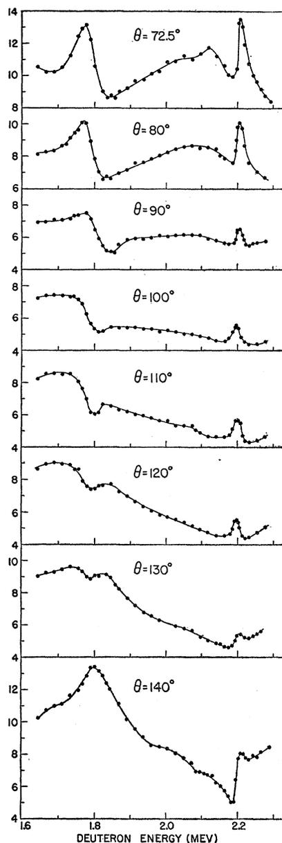
FIG. 5. Excitation curves for the  $C^{13}(d,\alpha)B^{11}$  (ground-state) reaction as a function of the bombarding energy in the vicinity of the 1.80- and 2.20-Mev resonances at 8 observation angles from  $72.5^\circ$  to  $180^\circ$ . The thin target was used so that the corrections for target thickness are negligible.
