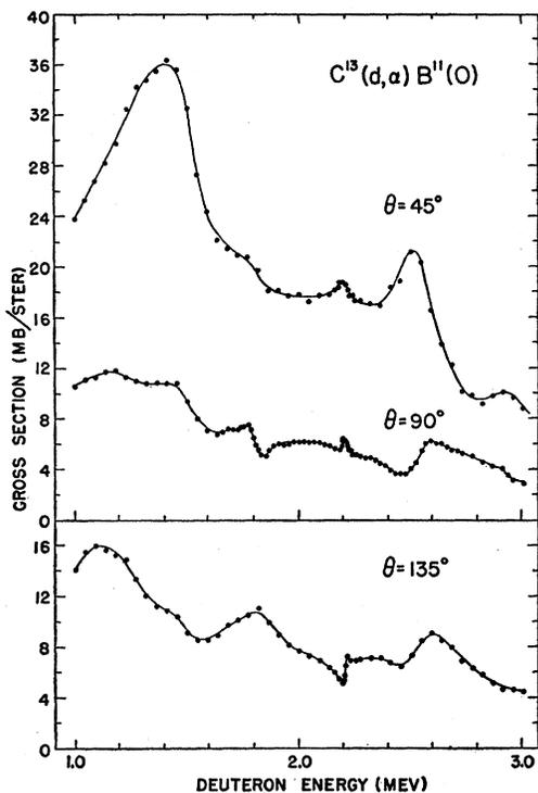
FIG. 3. Excitation curves for the  $C^{13}(d,\alpha)B^{11}$  (ground state) reaction as a function of the bombarding energy at observation angles of  $45^\circ$ ,  $90^\circ$ , and  $135^\circ$ . The foil target was used and the energy scale is uncorrected for target thickness.
