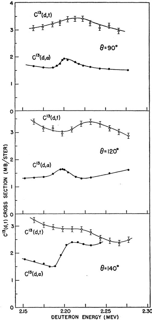
FIG. 8. Excitation curves for the  $C^{13}(d,t)C^{12}$  (ground-state) reaction as a function of the bombarding energy in the vicinity of the 2.20-Mev resonance. The curves for the  $C^{13}(d,\alpha)$  reaction are the same as those shown in Fig. 5 and have been included for purposes of comparison. The thin target was used so that corrections for target thickness are negligible. The indicated differential cross sections are for the  $(d,t)$  reaction only.
