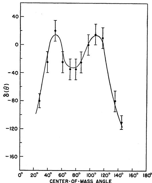
FIG. 11. Relative phase between the resonant and nonresonant parts of the cross section at the 2.20-Mev resonance in the  $C^{13}(d,\alpha)B^{11}$  (ground-state) reaction.
