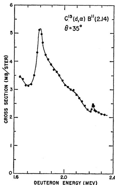
FIG. 7. Excitation curve for the  $C^{13}(d,\alpha)B^{11}(2.14)$  reaction as a function of the bombarding energy in the vicinity of the 1.80- and 2.20-Mev resonances. The foil target was used and the energy scale is uncorrected for target thickness.
