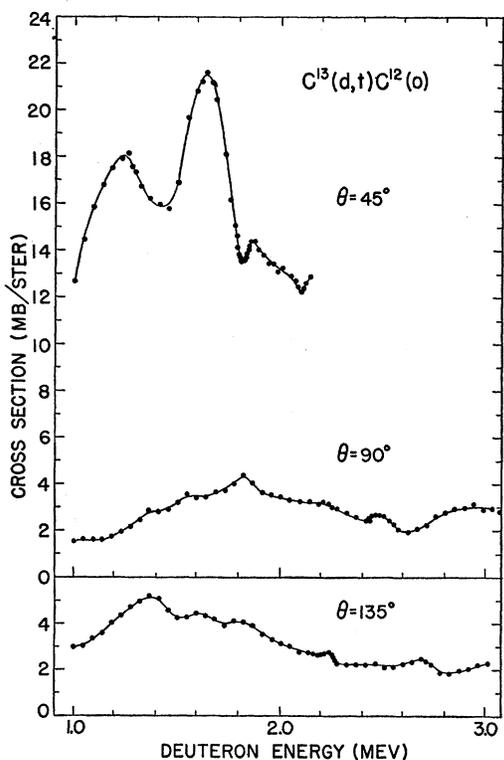
FIG. 4. Excitation curves for the  $C^{13}(d,t)C^{12}$  (ground state) reaction as a function of the bombarding energy at observation angles of  $45^\circ$ ,  $90^\circ$ , and  $135^\circ$ . The foil target was used and the energy scale is uncorrected for target thickness.
