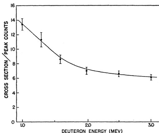
FIG. 2. Empirical correction curve relating the peak counts in a momentum profile to the differential cross section. The curve is for the ground-state  $\alpha$  particles and tritons from  $C^{13}+d$  and was obtained with the foil target.
