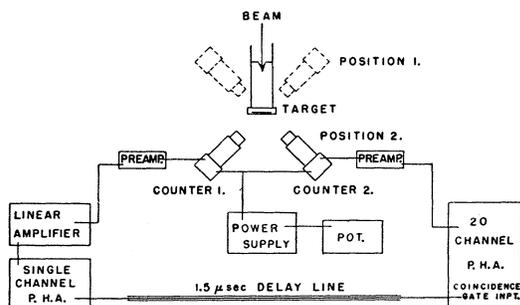
FIG. 3. Schematic diagram of experimental arrangement for detection of coincidence  $\gamma$ -ray spectra. Position 1 gave somewhat better resolution but with some reduction in counting rate.
