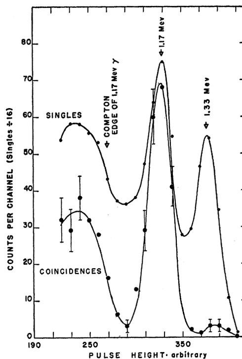
FIG. 4. Test coincidence spectrum taken with a  $\text{Co}^{60}$  source. The 1.33-Mev radiation was used to gate the 20-channel analyzer which recorded the coincidence spectrum shown. The singles spectrum is shown for comparison.
