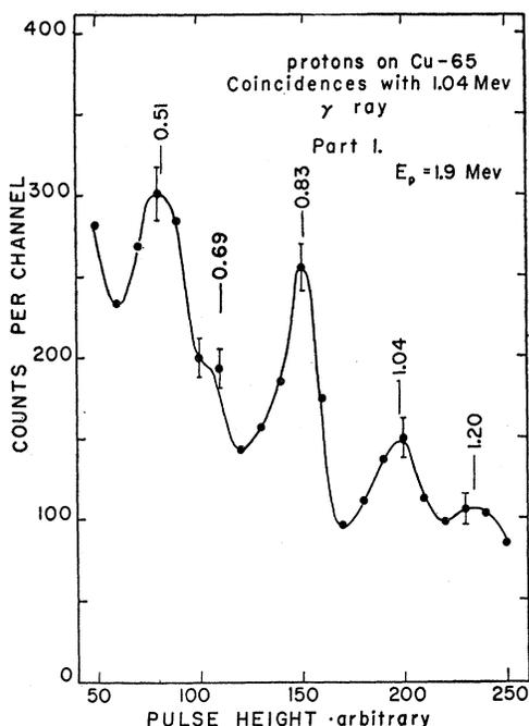
FIG. 7. The energy spectrum of  $\gamma$  rays in the interval 0–1.3 Mev which are in coincidence with the 1.04-Mev  $\gamma$  ray observed when  $\text{Cu}^{65}$  is bombarded with 1.9-Mev protons.
