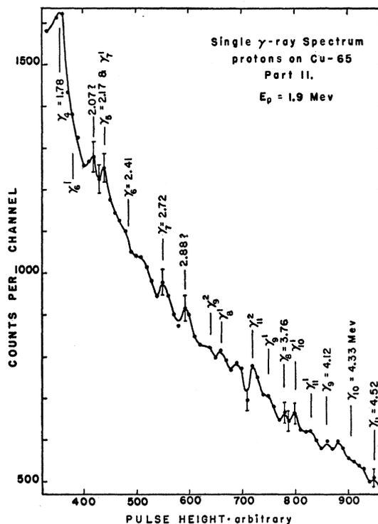
FIG. 6. The energy spectrum of  $\gamma$  rays in the interval 1.7–4.6 Mev observed when  $\text{Cu}^{65}$  is bombarded with 1.9-Mev protons.  $\gamma_i$  = photopeak;  $\gamma_i^1$  = pair production with escape of one annihilation photon;  $\gamma_i^2$  = pair production with escape of both annihilation photons.
