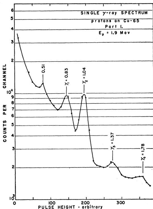
FIG. 5. The energy spectrum of  $\gamma$  rays in the interval 0–1.8 Mev observed when  $\text{Cu}^{65}$  is bombarded with 1.9-Mev protons.  $\gamma_i$  indicates the photopeak of a given  $\gamma$  ray.
