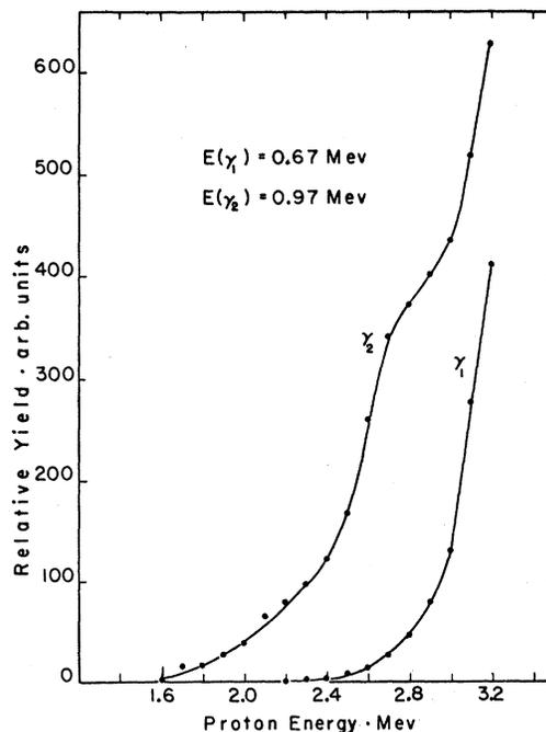
FIG. 16. Thick-target yield of the 0.67-Mev and 0.97-Mev γ rays observed when Cu<sup>63</sup> is bombarded with protons.
