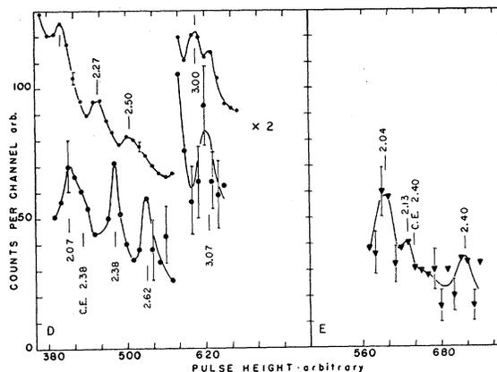
FIG. 13. Various 20-channel spectra of the  $\gamma$  rays in coincidence with the 0.97-Mev  $\gamma$  ray observed when  $\text{Cu}^{63}$  is bombarded with 2.5-Mev protons.  $\blacktriangledown$ — position 1 (see Fig. 3);  $\blacktriangle$ — repeated spectrum, position 1;  $\bullet$ — position 2. Singles spectra are plotted at the top for comparison purposes.
