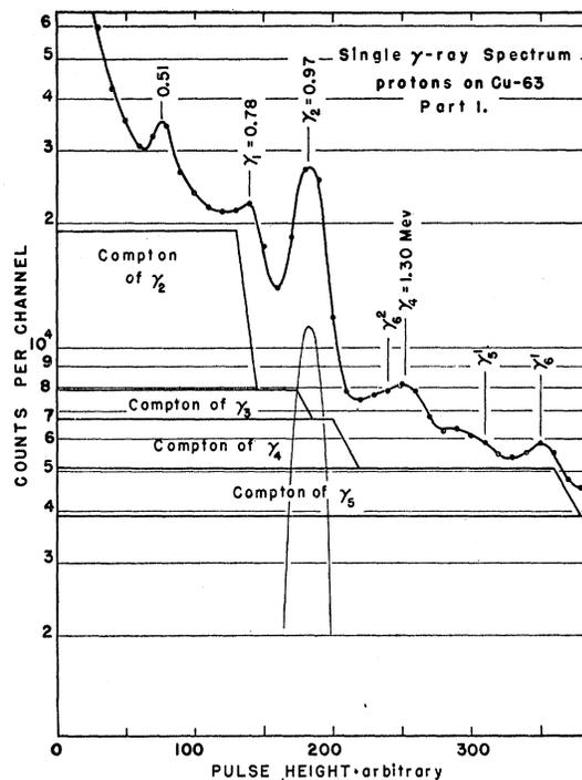
FIG. 10. The energy spectrum of γ rays in the interval 0-1.8 Mev observed when Cu<sup>63</sup> is bombarded with 2.0-Mev protons. γ<sub>i</sub>=photopeak; γ<sub>i</sub><sup>1</sup>=pair production with escape of one annihilation photon; γ<sub>i</sub><sup>2</sup>=pair production with escape of two annihilation photons. Resolution of the spectrometer is indicated at intervals.
