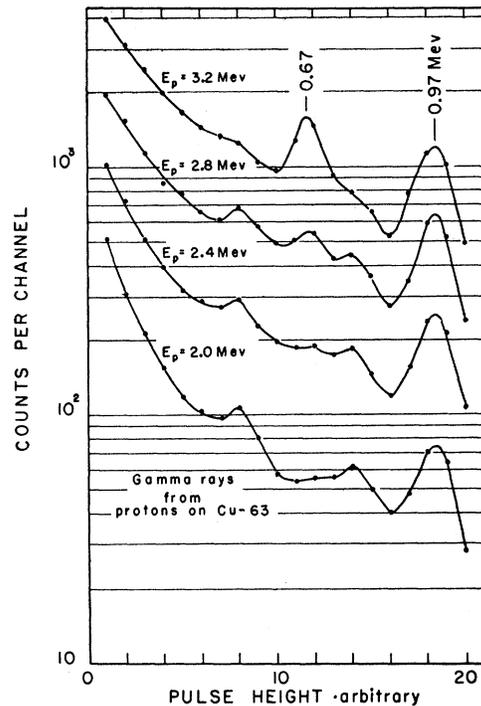
FIG. 15. The spectra of gamma rays from Cu<sup>63</sup> when bombarded with protons of various energies.
