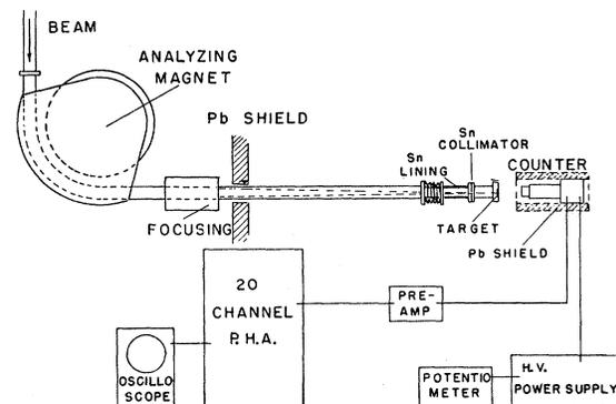
FIG. 1. Schematic diagram of experimental arrangement for detection of single  $\gamma$ -ray spectra.
