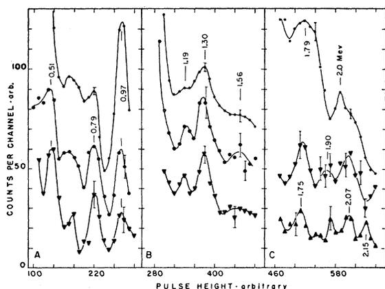
FIG. 12. Various 20-channel spectra of the  $\gamma$  rays in coincidence with the 0.97-Mev  $\gamma$  ray observed when  $\text{Cu}^{63}$  is bombarded with 2.5-Mev protons.  $\blacktriangledown$ — position 1 (see Fig. 3);  $\blacktriangle$ — repeated spectrum, position 1;  $\bullet$ — position 2. Singles spectra are plotted at the top for comparison purposes.
