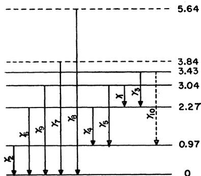
FIG. 14. The proposed decay scheme of Zn<sup>64</sup> which is formed by proton capture in Cu<sup>63</sup>. Energies are in Mev. Dotted levels and transitions are uncertain.
