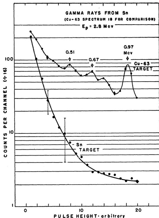
FIG. 2. Pulse-height spectrum of the  $\gamma$  rays from tin bombarded with 2.8-Mev protons. The spectrum of  $\gamma$  rays from  $\text{Cu}^{63}$  is shown for comparison.
