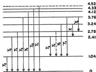
FIG. 9. The proposed decay scheme of  $\text{Zn}^{66}$  which is formed by proton capture in  $\text{Cu}^{65}$ . Energies are in Mev. Dotted levels and transitions are uncertain.
