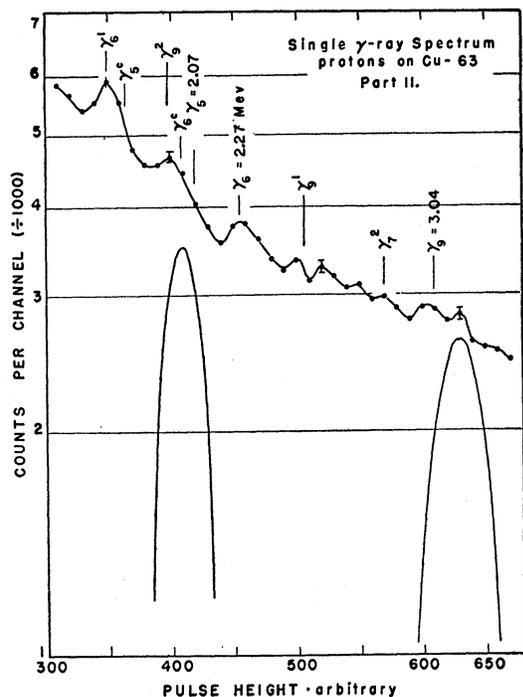
FIG. 11. The energy spectrum of  $\gamma$  rays in the interval 1.6–3.2 Mev observed when  $\text{Cu}^{63}$  is bombarded with 2.0-Mev protons.  $\gamma_6$ =photopeak;  $\gamma_4^1$ =pair production with escape of one annihilation photon;  $\gamma_4^2$ =pair production with escape of two annihilation photons. Resolution of the spectrometer is indicated at intervals.
