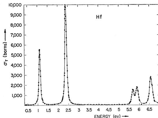
FIG. 1. The total neutron cross section of hafnium.
