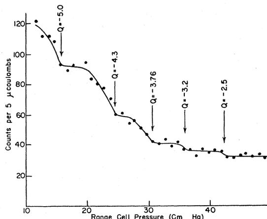
FIG. 8. Slow-neutron threshold curve for the reaction  $F^{19}(\alpha, n)Na^{22}$ .
