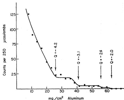
FIG. 7. Integral range curve for the reaction  $F^{19}(\alpha, n)Na^{22}$ .
