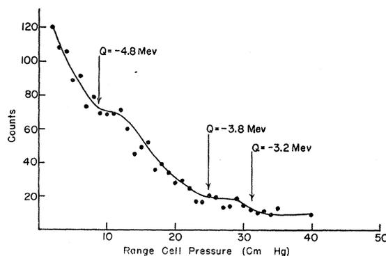
FIG. 6. Slow-neutron threshold curve for the reaction  $B^{11}(\alpha,n)N^{14}$ .
