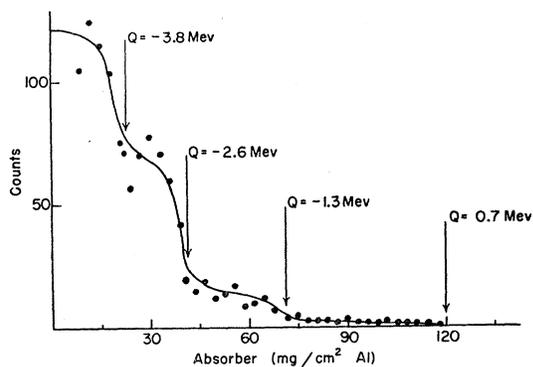
FIG. 3. Integral range curve for the reaction  $B^{10}(\alpha,n)N^{13}$ .
