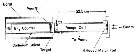
FIG. 2. The slow-neutron threshold detector.
