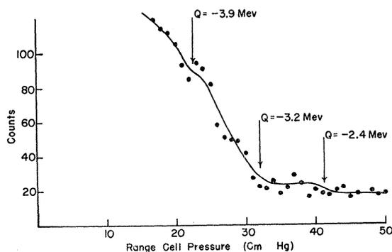
FIG. 4. Slow-neutron threshold curve for the reaction  $B^{10}(\alpha,n)N^{13}$ .
