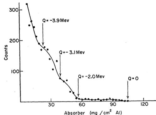
FIG. 5. Integral range curve for the reaction  $B^{11}(\alpha,n)N^{14}$ .
