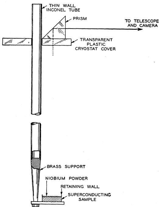
Fig. 2. Apparatus for observing intermediate state domain patterns.
