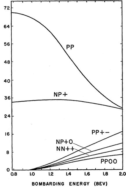
FIG. 7. The relative probability for the occurrence of  $p$ - $p$  initiated two- and four-pronged events as a function of the bombarding energy. Curves are labeled by the charges of the final particles.
