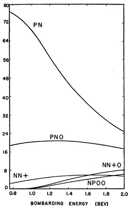
FIG. 8. The relative probability for the occurrence of  $n$ - $p$  initiated one-pronged events as a function of the bombarding energy. The curves are labeled by the charges of the final particles resulting from the collision.
