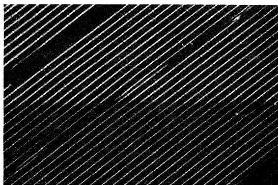
FIG. 2. An interferogram of an x-rayed crystal. The lower part of the crystal has been irradiated (50X).
