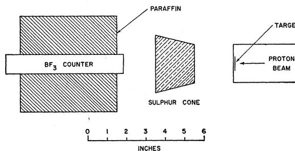
FIG. 1. Geometrical arrangement of the neutron detector and absorber sample used for making the transmission measurements.
