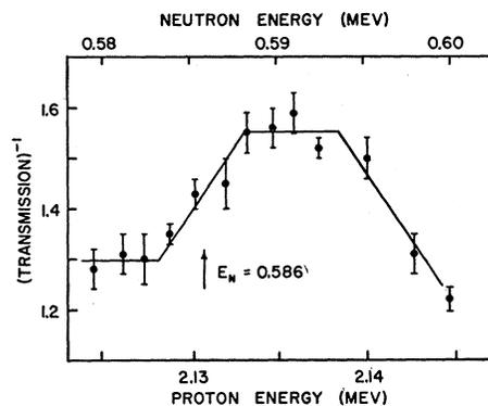
Fig. 3. Reciprocal of the transmission through a sulfur sample as a function of proton energy for neutrons from the  $\text{V}^{51}(p,n)\text{Cr}^{51}$  reaction. The indicated probable errors are the standard deviations for a number of determinations at each energy.
