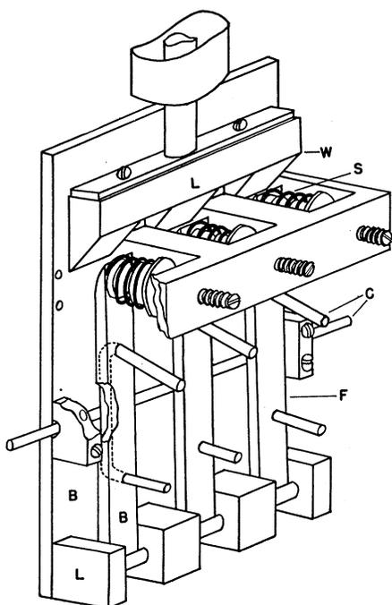
FIG. 1. Mount for crossed-wire contacts. The Lucite wedge (W) is inserted under the flaps (F), holding the contact wires (C) against the force of the springs (S). The wedge is withdrawn when contact is desired. Brass parts are designated by (B), Lucite by (L).
