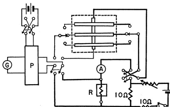
FIG. 2. Electrical circuit for measuring contact resistance. G: Leeds & Northrup Galvanometer, model HS 2284-b. P: L & N Potentiometer model K-2. R: Wolff 1-international-ohm standard resistor. A: Simpson model 373 milliammeter. The parts enclosed by dashed lines are at liquid helium temperature.
