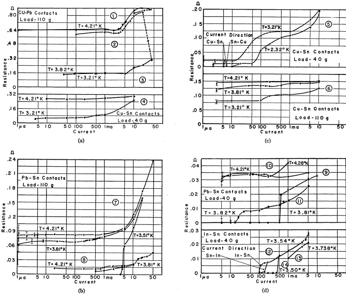
FIG. 3. Plots of observed resistance *vs* current for contacts between crossed wires of normal conducting metals and superconducting metals.
