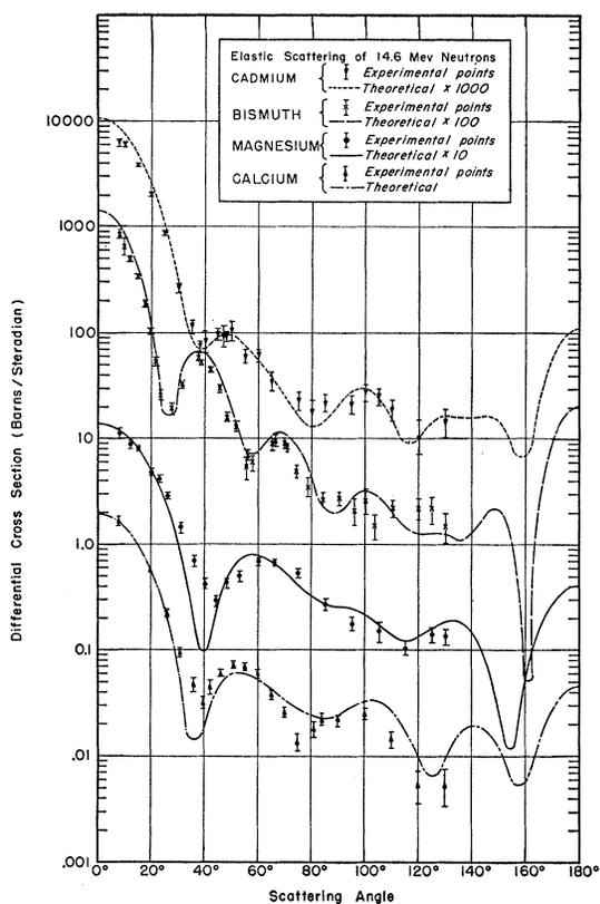
FIG. 2. The angular distributions for magnesium, calcium, cadmium, and bismuth—experimental and computed.
