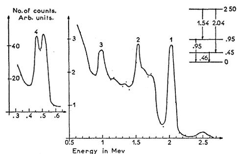
FIG. 1.  $\gamma$  spectrum of the yield from the 222-keV resonance and decay scheme for the 2.50-MeV level.
