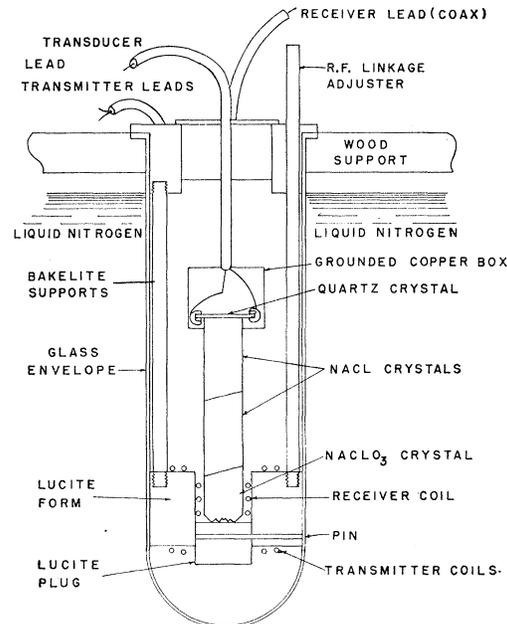
FIG. 4. The arrangement of the transducer and nuclear induction head.
