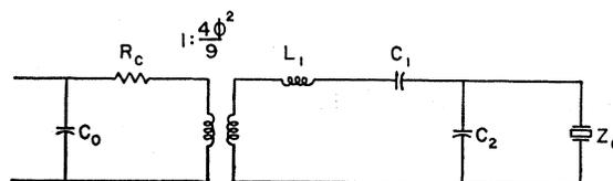
Fig. 8. The equivalent circuit of the quartz transducer.
