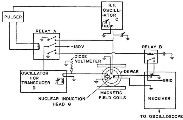
FIG. 3. A block diagram of the equipment.
