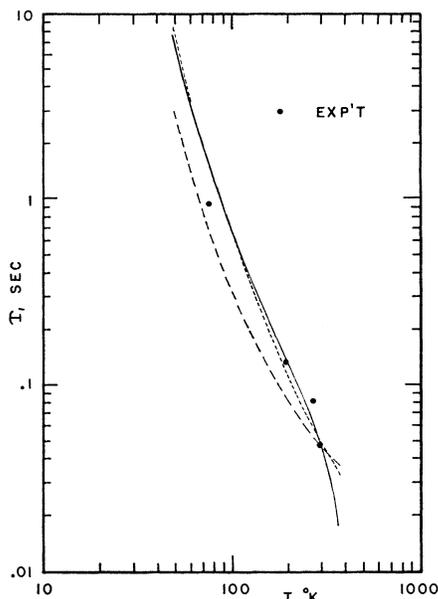
FIG. 5. The circles show the experimentally observed relation between the thermal relaxation time and the temperature for  $\text{NaClO}_3$  crystals. The lines represent the theoretical predictions of Chang using various assumptions.<sup>6</sup>
