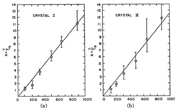
FIG. 7. (a) The relation between  $x = (T_1/T_{1b})$  (ordinate) and  $T_p^{-1}$  times the energy density in ergs/cm<sup>3</sup> for crystal I (abscissa).  $T_p$  is the phonon relaxation time. (b) The same data for crystal II.
