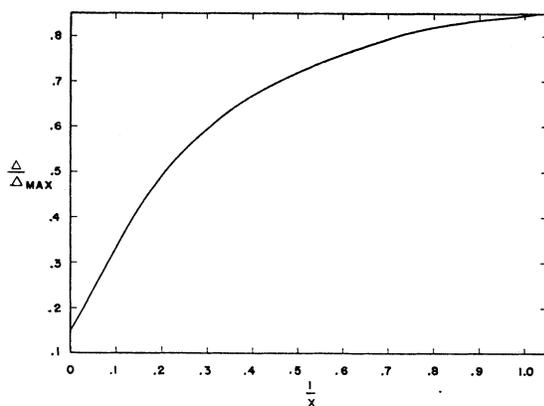
FIG. 6. The predicted relation between the quantities  $\Delta/\Delta_{\max}$  and  $1/x$ , where  $\Delta$  is the population difference with ultrasonic excitation present and  $\Delta_{\max}$  is the population difference without the ultrasonic present.  $x = T_1/T_{1b}$ , where  $T_1$  is the thermal relaxation time without the ultrasonic excitation present and  $T_{1b}$  is the contribution to the relaxation due to the ultrasonic excitation.
