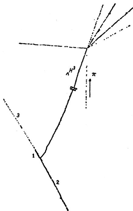
FIG. 5. Event 89 was found in a pellicle exposed to 3-Bev  $\pi^-$  mesons. The hyperfragment,  $\Lambda H^3$ , traveled 324 microns and decayed into three coplanar particles; a  $\pi^-$  meson of 23.4 Mev (track 3), a deuteron (track 1), and a proton (track 2).
