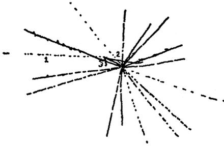
FIG. 6. The hyperfragment was produced by cosmic rays in pellicles aligned for a  $K^-$ -exposure. Hence none of the tracks could be followed. The three tracks from the hyperfragment decay are not coplanar. The energy of the  $\pi^-$  meson (track 1) is 25.5 Mev from the grain density. If tracks 2 and 3 were due to a proton and deuteron, respectively, the binding of the  $\Lambda$  particle in  $\Lambda H^4$  is  $1.9 \pm 2.0$  Mev.
