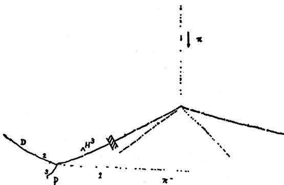
FIG. 4. A drawing of event 87. The three tracks from the hyperfragment are coplanar. Track 1 is 1.71 cm long and due to a  $\pi^-$  meson. Momentum is balanced if tracks 2 and 3 are assigned to a deuteron and a proton, respectively. The binding of the  $\Lambda^0$  particle in  $\Delta H^3$  is found to be  $0.6 \pm 0.6$  Mev.
