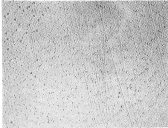
FIG. 4. Random dislocations in germanium crystal. CP<sup>4</sup> etch, 500X. Approximate density,  $10^5$  dislocations per cm<sup>2</sup>. Area reduced approximately 66% in reproduction.
