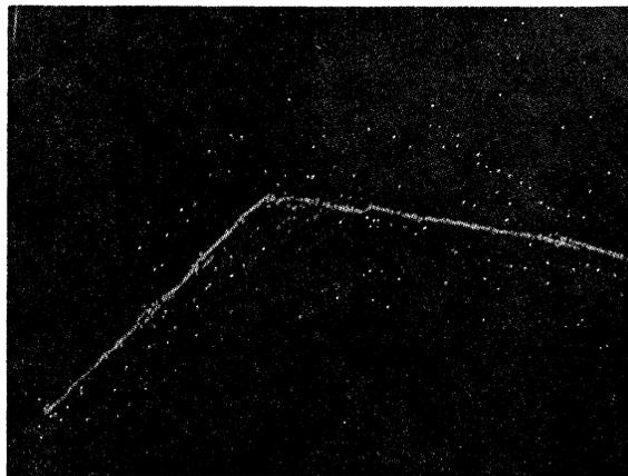
FIG. 1. Low-angle boundary in germanium, electropolished and etched, dark field, 100X. Area reduced approximately 66% in reproduction.
