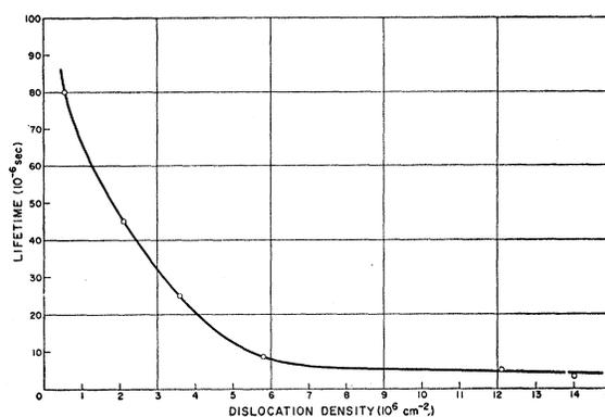
FIG. 9. Dislocation density vs lifetime for silicon.
