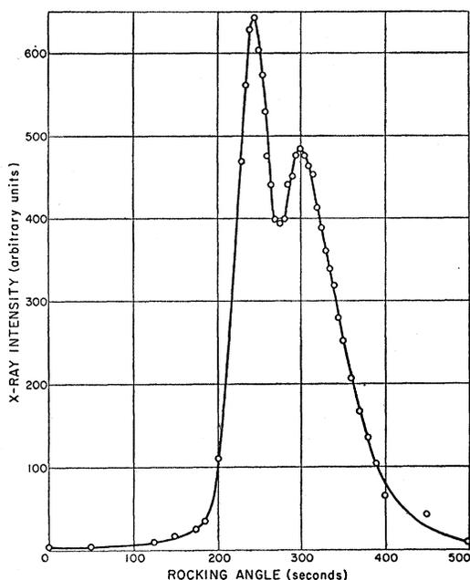
FIG. 2. Rocking curve with x-ray beam straddling boundary (111) reflection. Misorientation across boundary approximately 80 seconds.
