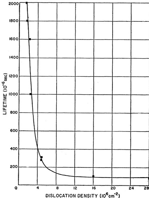
FIG. 7. Dislocation density *vs* lifetime for low-resistivity germanium.
