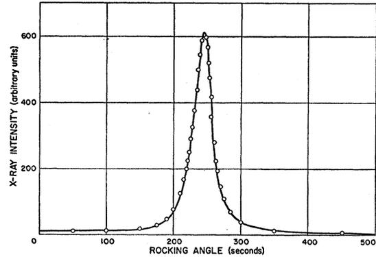
FIG. 5. Typical rocking curve for germanium. Cu  $K\alpha$  radiation.
