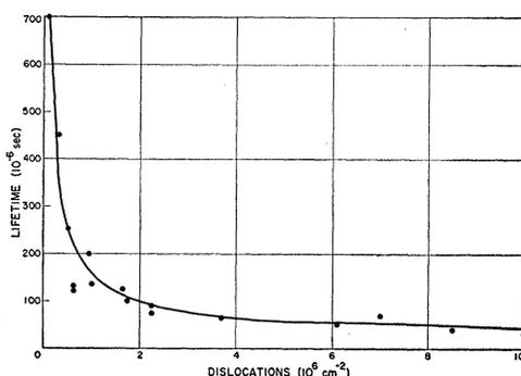
FIG. 8. Dislocation density vs lifetime for high-lifetime germanium.
