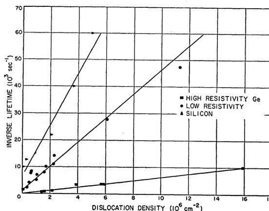
FIG. 10. Dislocation density vs inverse lifetime.
