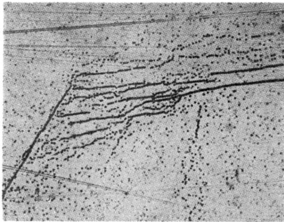
FIG. 3. Dislocation geometry near intersection of low-angle boundaries. Electropolished and etched, 100X. Area reduced approximately 66% in reproduction.
