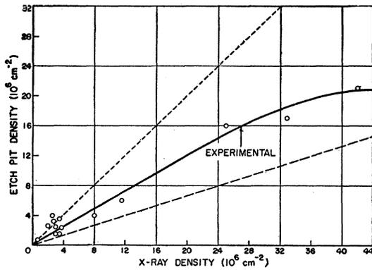
FIG. 6. Comparison of etch pit and x-ray dislocation density.
