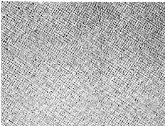
FIG. 4. Random dislocations in germanium crystal. CP<sup>4</sup> etch, 500X. Approximate density,  $10^6$  dislocations per cm<sup>2</sup>. Area reduced approximately 66% in reproduction.
