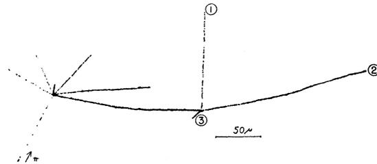
FIG. 5. Decay of  ${}^5\text{He}^{5*}$  hyperfragment ejected from a 6-prong star produced by 1.5-Bev pion.
