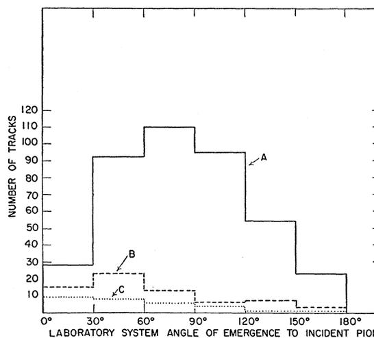
FIG. 3. Angular distributions of tracks emerging from 1.5-Bev pion-produced stars: A, outgoing black tracks; B, outgoing grey tracks; C, outgoing minimum tracks.
