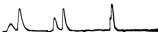
FIG. 3. Sweep triggered by fission-chamber pulse. Left to right: fission pulse, prompt tank pulse from fission \gamma rays and recoil protons, and four neutron-capture pulses.
