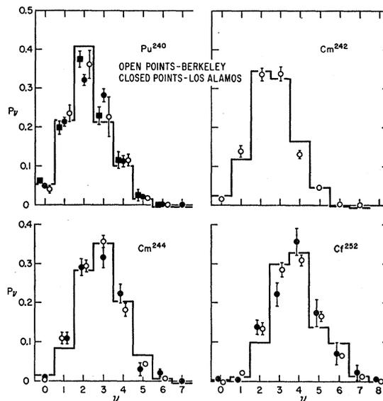
FIG. 4. Neutron emission probabilities for spontaneous fission. Calculated results are given by lines. Data are: open circles, Hicks *et al.*; closed circles, Diven *et al.*; and squares, Hammel and Kephart.
