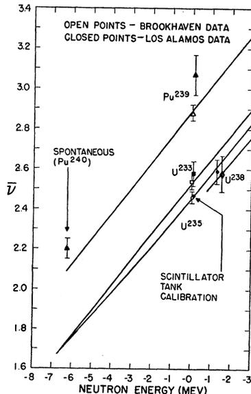
FIG. 5. Variation of  $\bar{\nu}$  with the energy of neutron inducing fission. Lines are calculations based on the method of Fowler and normalized to  $E_n = 0$  measured values. Los Alamos data are of Diven *et al.*; Brookhaven data are from BNL-325.
