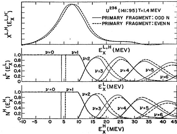
FIG. 2. Calculated excitation energy distributions,  $X^L$  and  $X^H$ , and neutron emission probabilities,  $N^L$  and  $N^H$ , for the most probable fission mode of thermal-neutron fission of  $U^{236}$  (compound nucleus  $U^{236}$ ). The abscissa scales for the three sets of curves are the same.
