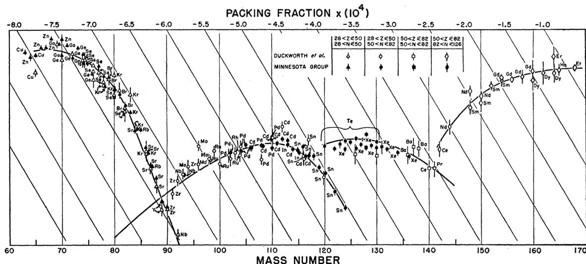
FIG. 1. The valley of the mass surface. The data shown are the results of conversions of the mass-spectrographic values to those of odd mass number and of the noninteger stable charge of the isobar.
