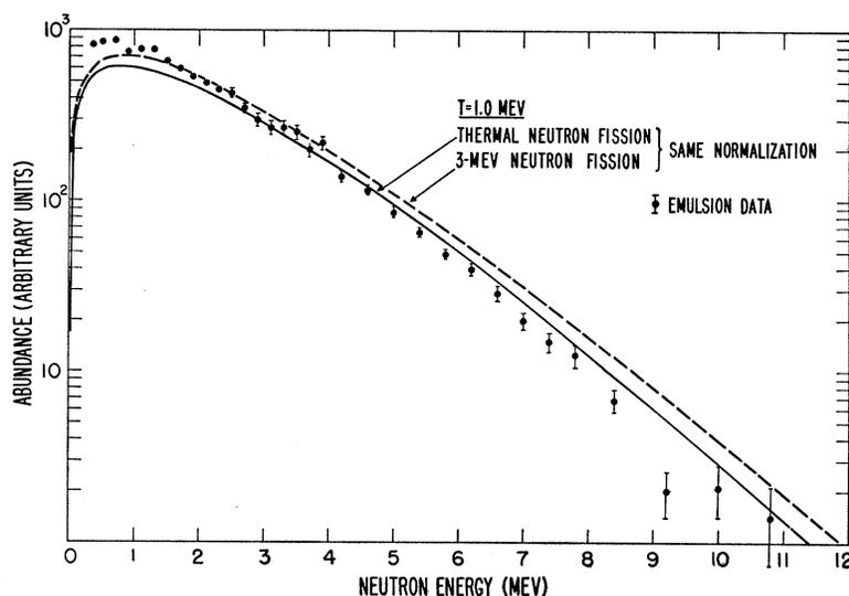
FIG. 6. Calculations of the energy spectra of fission neutrons for  $T=1.0$  Mev. Data are of Frye and Rosen.
