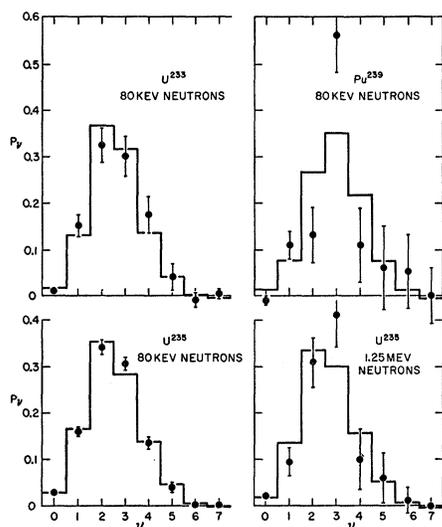
FIG. 3. Neutron emission probabilities for neutron-induced fission. Calculated results are given by lines. Circles are the data of Diven *et al.*
