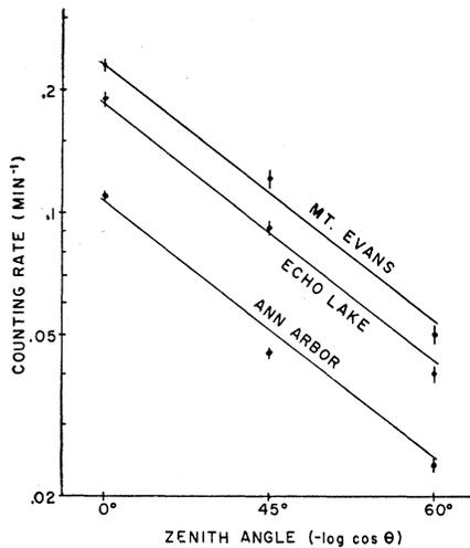
Fig. 2. Zenith-angle dependence of penetrating particles. The straight lines are proportional to  $\cos^{2.10}$ .
