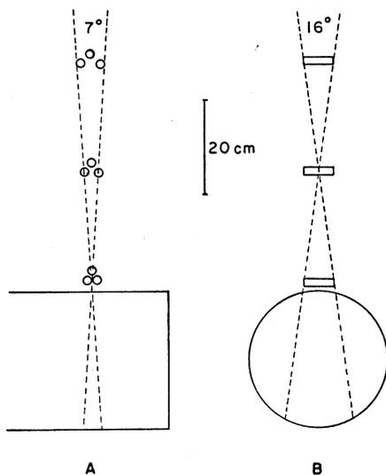
FIG. 1. Arrangement of counters and cloud chamber. A. Side view. B. Front view.
