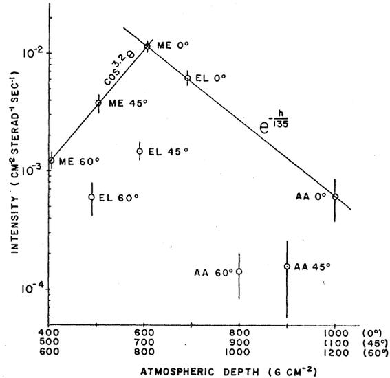
FIG. 5. Intensities of electrons with  $E > 10$  Mev resulting from nuclear interactions, plotted against atmospheric depth. The points for zenith angle  $45^\circ$  are offset by  $100 \text{ g cm}^{-2}$  to the left, and the points for  $60^\circ$  are offset by another  $100 \text{ g cm}^{-2}$ . For a given altitude the graph may be considered as a plot of intensity against  $-\log \cos\theta$ .
