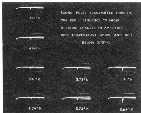
FIG. 3. Photographs of oscilloscope—3.64 to 4.15°K.
