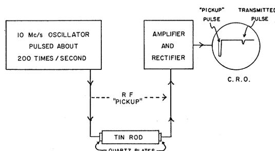
FIG. 1. Block diagram of the experimental arrangement.
