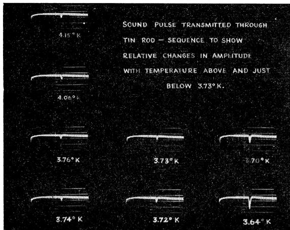
FIG. 3. Photographs of oscilloscope—3.64 to 4.15°K.
