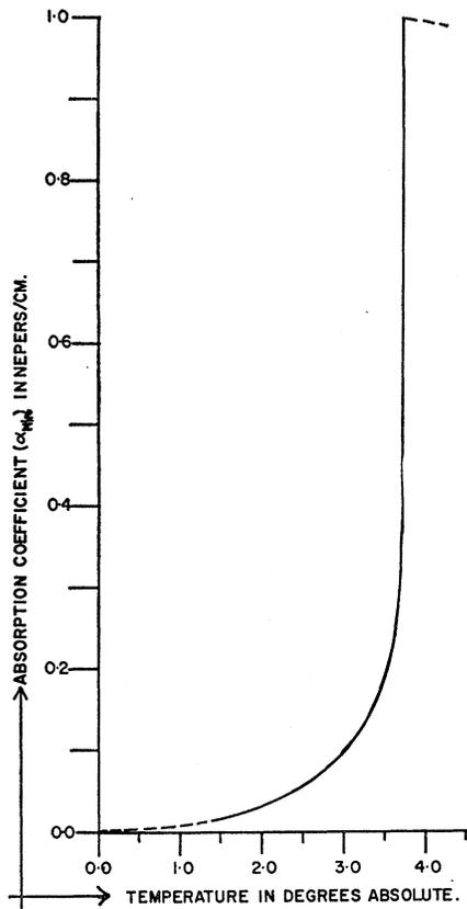
FIG. 6. Graph of the electronic absorption coefficient ( $\alpha_{T \min}$ ) plotted against absolute temperature.
