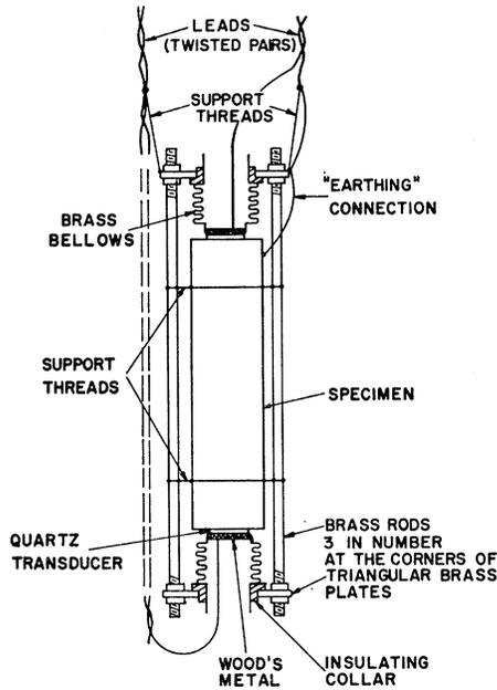
FIG. 2. Experimental arrangement for mounting the tin specimen.
