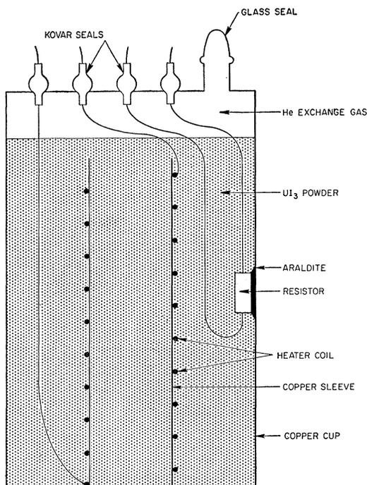
FIG. 3. Calorimeter cup assembly for specific heat measurements.
