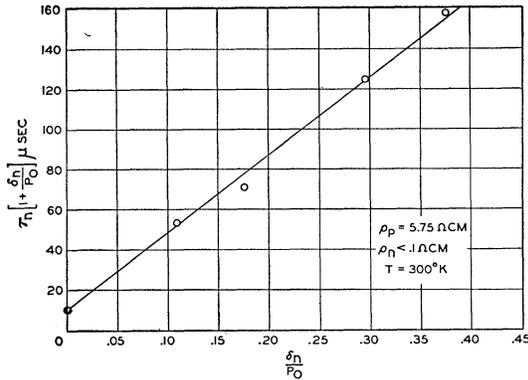
FIG. 2. Lifetime in *p*-type silicon vs injected electron density.
