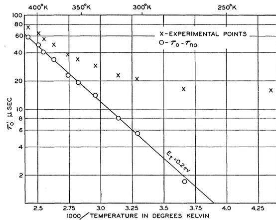
FIG. 3. Lifetime in 20 $\Omega$ -cm *p*-type silicon vs 1000/*T*. The slope of  $\tau_0 - \tau_{n0}$  gives the level of recombination centers within the energy gap.
