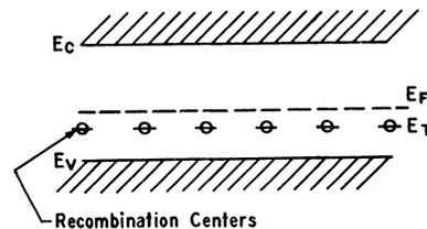
FIG. 1. Model for the recombination of electrons and holes.
