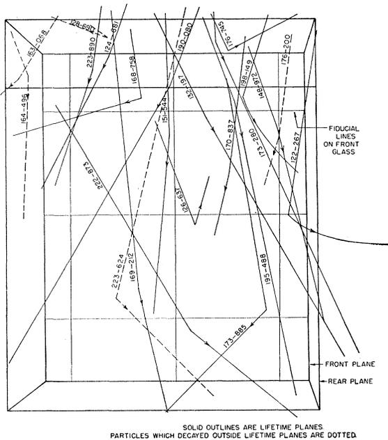
FIG. 7. Fiducial planes used for lifetime measurements.
