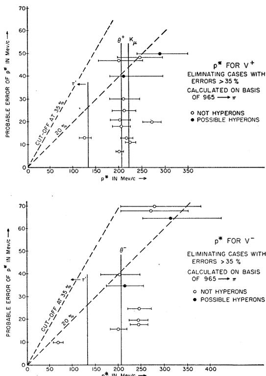
FIG. 5. Momenta of the charged secondaries in the c.m. system for  $V^+$  and  $V^-$  events. These are plotted in order of increasing probable error in the momenta. The cut-off lines determine quickly how many events are eliminated by making the percentage error requirements more stringent.
