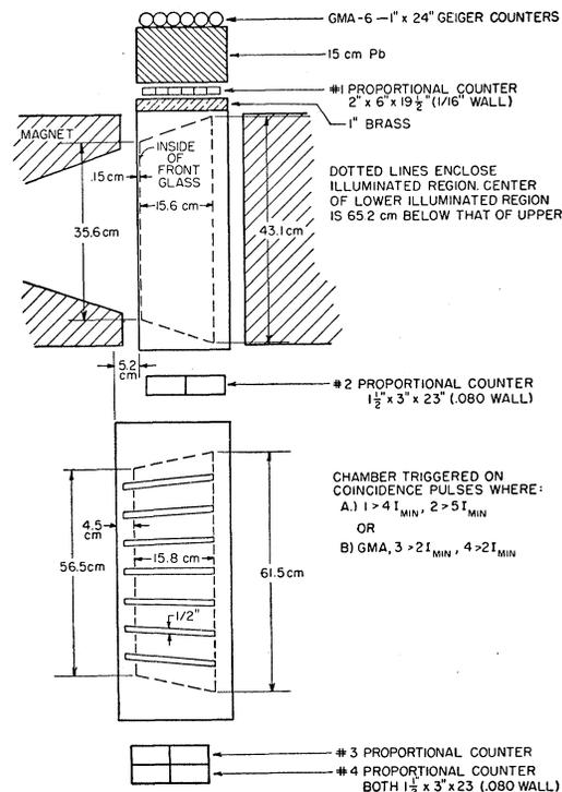
FIG. 1. Experimental arrangement for dual cloud chambers. This is presented as a typical arrangement. However, the counter disposition and depth of illumination has been varied during the course of the experiment.
